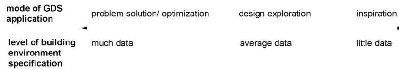
Figure 31. Three ways of applying the generative design system. In a well-specified building environment, the GDS works as a problem solver. In an undefined building environment, the GDS works as a generator of forms for inspiration. The intermediary position is the most typical: there is an average amount of data and the GDS can be used for design exploration.
