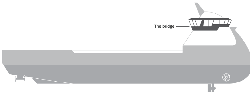
Figure 4: The bridge of an OSV is typically positioned at the top deck at the front of the vessel. (Author's illustration, based on Ulstein's PX105 ship design)
