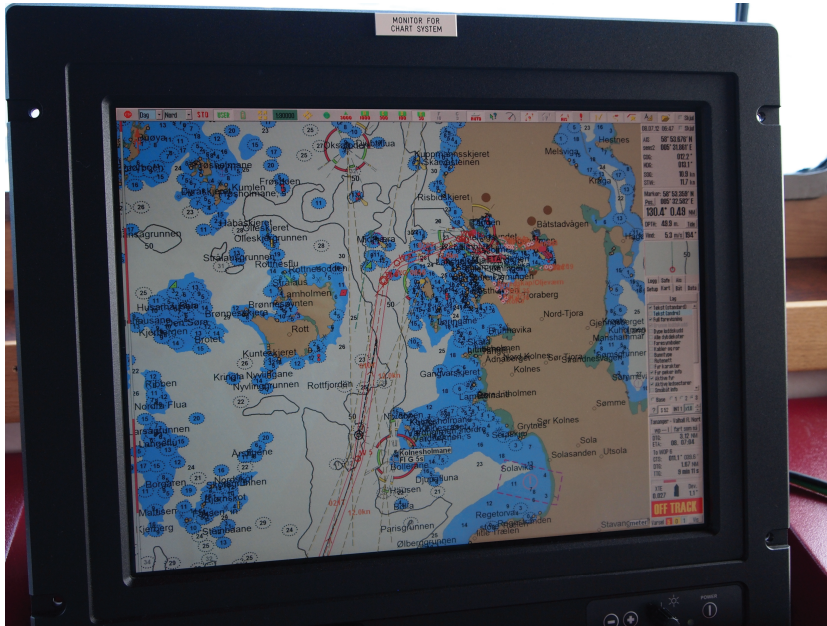
Figure 31: The electronic charts (ECDIS) stood out in the field studies as a system that the deck officers found hard to use beyond the basic functionality. (Photo: UBC)
