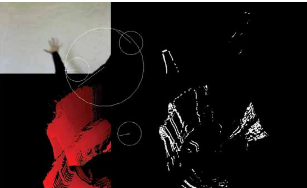
Figure 3.2d A screenshot of working in TKB's Arts lab with an openFrameworks (oF) example adapted in an oF workshop with Castro at the Art-on-Wires conference in Oslo in 2010. The application uses pixel comparison to calculate direction of boundaries (smaller circle) and of overall movement in the frame (larger circle).
