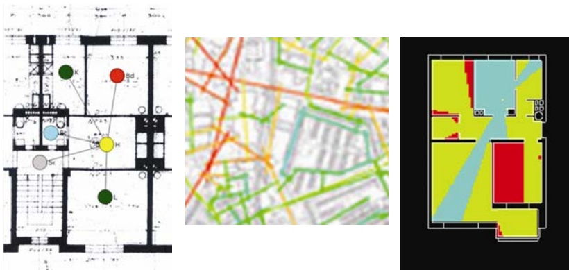
Figure 3.17 (a, b, c) The three modes of space syntax modelling: nodes, axial-lines and visual fields / isovists.
