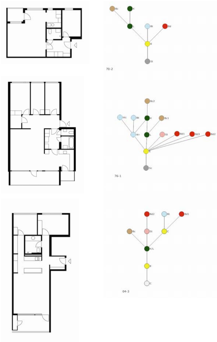
Figure 3.24 Examples of node-modelling, floor plans and space syntax connectivity graphs of 70-2, 76-1 and 04-3.
