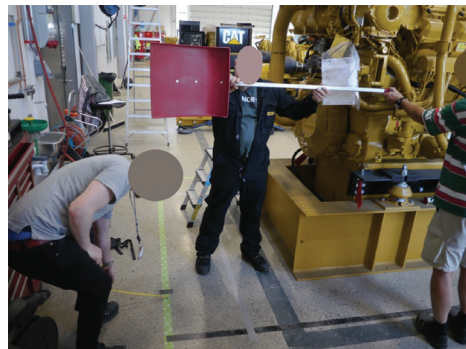
Figure 9. Space requirement capture for use-scenario: crankshaft removal. The crankshaft need to be pulled out entirely, requiring a lot of space.
