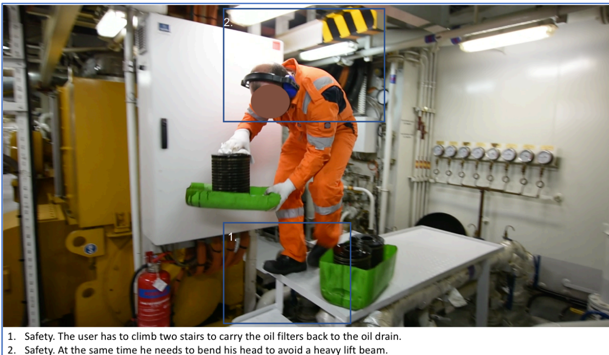
Figure 13 Step 3: example of presentation slide used in a collaborative data analysis workshop. In this case the observed scenario was the change of three oil filters on an engine.
