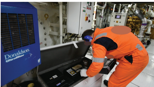
Figure 2. Service tools are stored in small boxes inside a larger box, making it inconvenient and time consuming for the operator to find the required tool. The lid of the tool box fell over the mechanic’s head during the operation.
