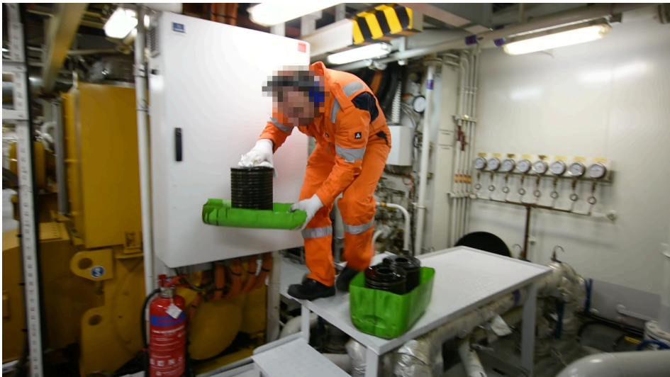
Figure 2: ONSITE Case #1: following a mechanic changing an oil filter in the engine room.
