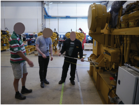
Figure 10. Space requirement capture for use-scenario: genset adjustment. The mechanic demonstrates the use of the tool required for this operation: a key with a long lever arm. To manipulate the key, the mechanic is standing one meter from engine.
