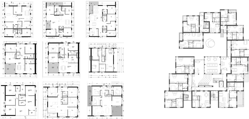
Figure 4.2 a) A wide range of choices for the 47 individual apartments at P1, where only load-bearing walls and main piping connection points are predefined. No group discussions among future neighbours. Drawing: Kaden + Lager. b) A limited number of choices for individual apartments at Vindmøllebakken, but extensive workshops and meetings to discuss and define the form of co-housing and to negotiate and plan the degree and type of shared features. Drawing: Helen & Hard. All drawings same scale.
