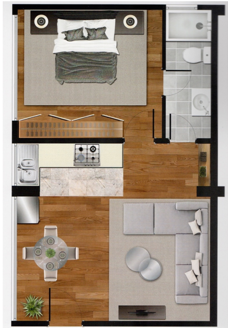
Figure 5.3 Floor plan of a one-bedroom apartment unit (54 square metres) in Kileleshwa showing the open plan typified by the absence of a full separating wall between the kitchen and the living room. (Vaal Real Estate, 2019, p. 26)
