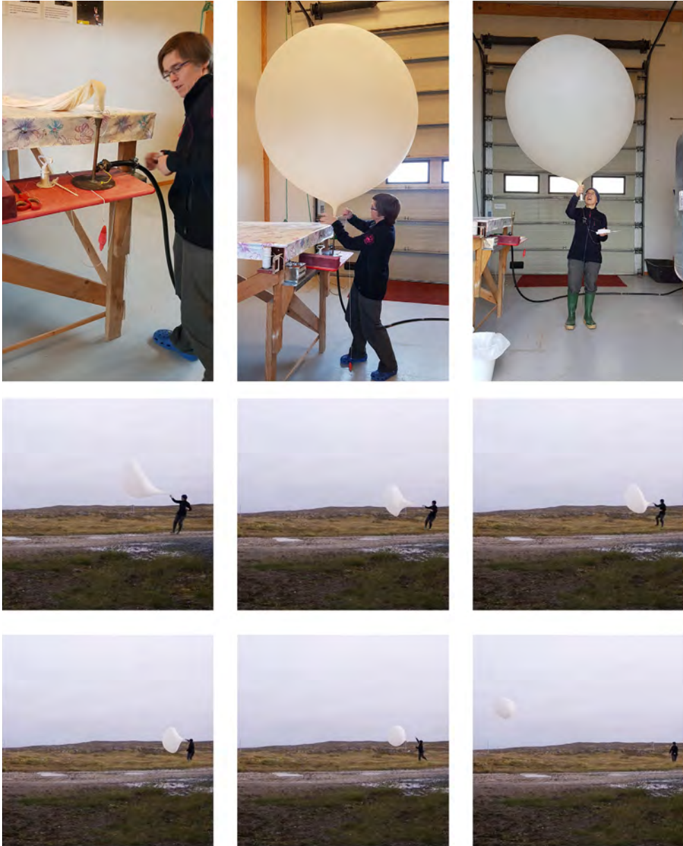
Fig.4.17. Balloon launch from Bjørnøya's meteorological station. The top three photographs show the preparation of the weather balloon (with a radiosonde attached to record weather data) by Venke Ivarrud. The six lower photographs show the stages of the balloon launch in very windy conditions. This balloon reached a height of 32,000m. Source: photograph by Eimear Tynan, 30 th August, 2018. Permission to reuse must be obtained from the rightsholder.
