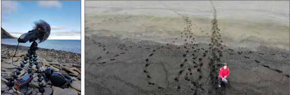
Fig.4.14. Equipment for audio recording. On the left is the audio recorder on a short tripod. Beside the recorder are a GPS device and headphones. The photograph on the right shows the tracks from a sound walk along Helenesanden, Jan Mayen. Source: photographs by Eimear Tynan, August, 2018. Permission to reuse must be obtained from the rightsholder.
