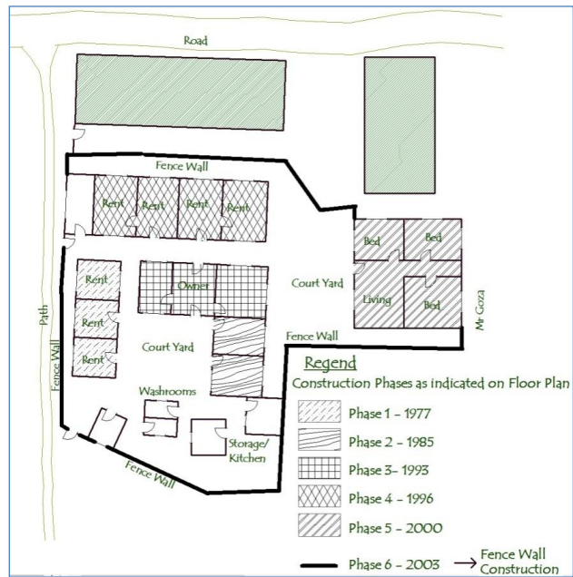
Figure 3.39: The completed house of Mr. Goza that comprised a series of rooms and fenced wall resulting from six construction phases that took about 26 years from 1977 to 2003.
