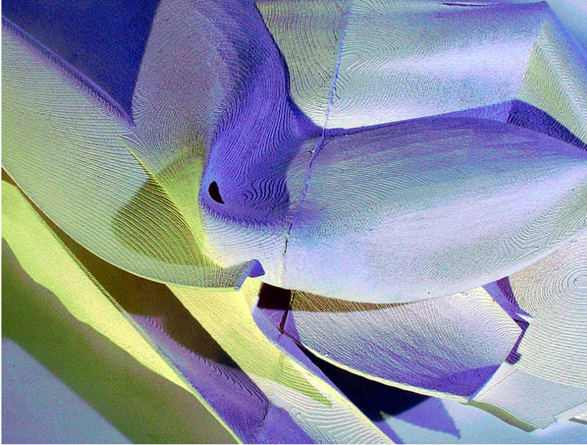
Figure 89 Emergent surface articulation from SLS production process. Synthetic Pavilion (Birger Sevaldson et al, 1997) This model was so complex that it was hard to understand on the screen only and the physical RP-model was necessary to investigate the emergent space fully. Polygonal file and the Selective Laser Sintering (SLS) left a pattern of surface articulation. The layers from the sintering produced a beautiful line pattern and the facets from the STL export file are barely visible as a secondary articulation.
