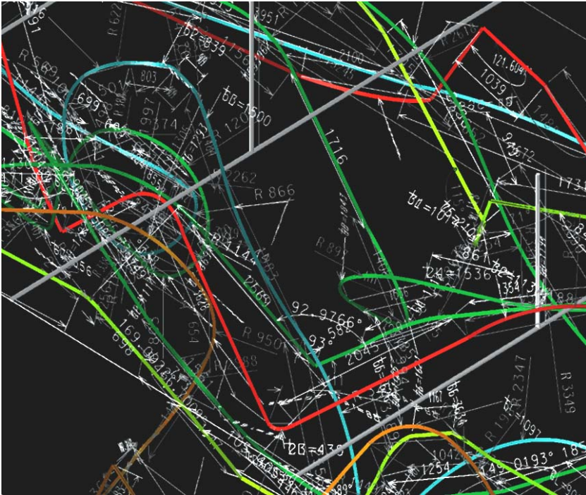
Figure 115 The digital model was rationalised by approximation of the NURBS geometries to fit with straight lines and circle segments. This allowed the production of simple construction drawings which were taken to a metal workshop for prefabrication of the elements. The result was rather imprecise and the elements were negotiated on site. This implied that the design process stretched into the construction of the installation. The modifications did not only imply “corrections” of imprecise geometries but on site consideration of the installation.
