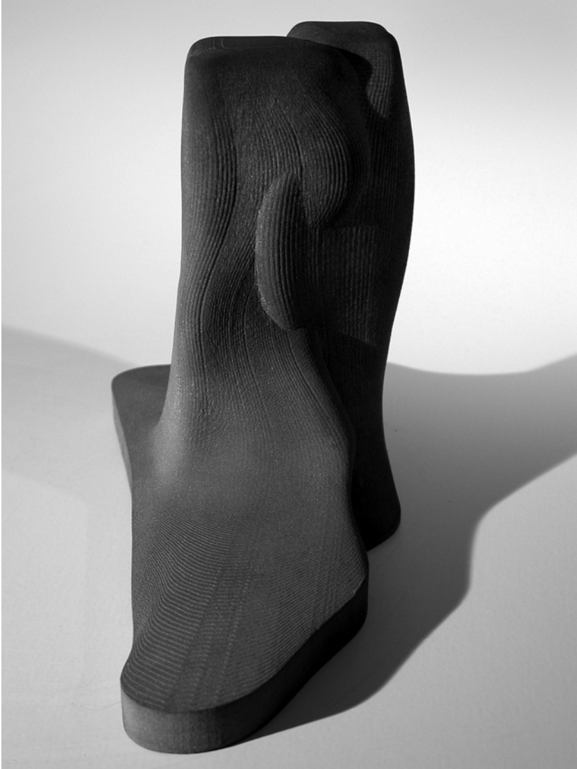
Figure 86 Rapid Form RP model of final solution. This is probably the first architectural model in this Steel / Bronze alloy rapid prototyping material from 3DSystems. The surface patterning indicating a façade design was made with displacement mapping challenging the borders of what was possible when it comes to the capacities of geometric construction and computational capacity.
