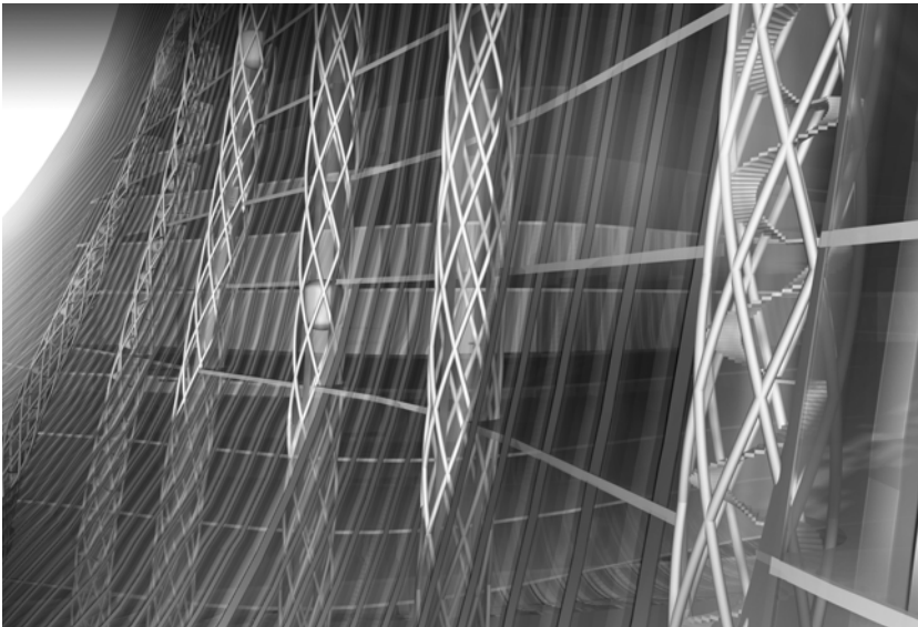
Figure 9 Detail of the façade showing the suggested networked system of vertical transportation channels and the striation of the façade.
