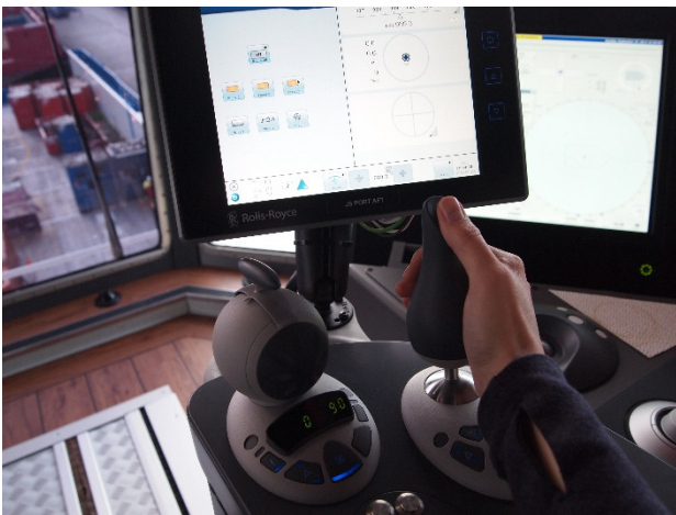
Figure 3: Testing what it feels like to sit in the DP (dynamic positioning) operator chair at a field study, September 2012 (Photo: UBC).
