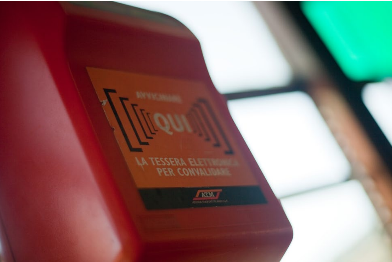
Figure 26: A 'RicaricaMI' RFID reader on the ATM transport network in Milan, Italy. The use of the term 'Qui' or 'Here' reveals the spatial aspects of RFID interaction.
