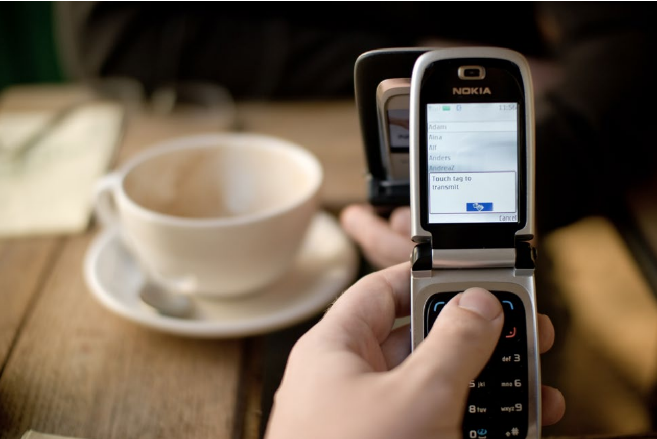
Figure 16: Using a variant of RFID, called Near Field Communication (NFC), in Nokia mobile phones to transfer contact data by bringing two handsets into close proximity, so called ‘Touch to transmit’.
