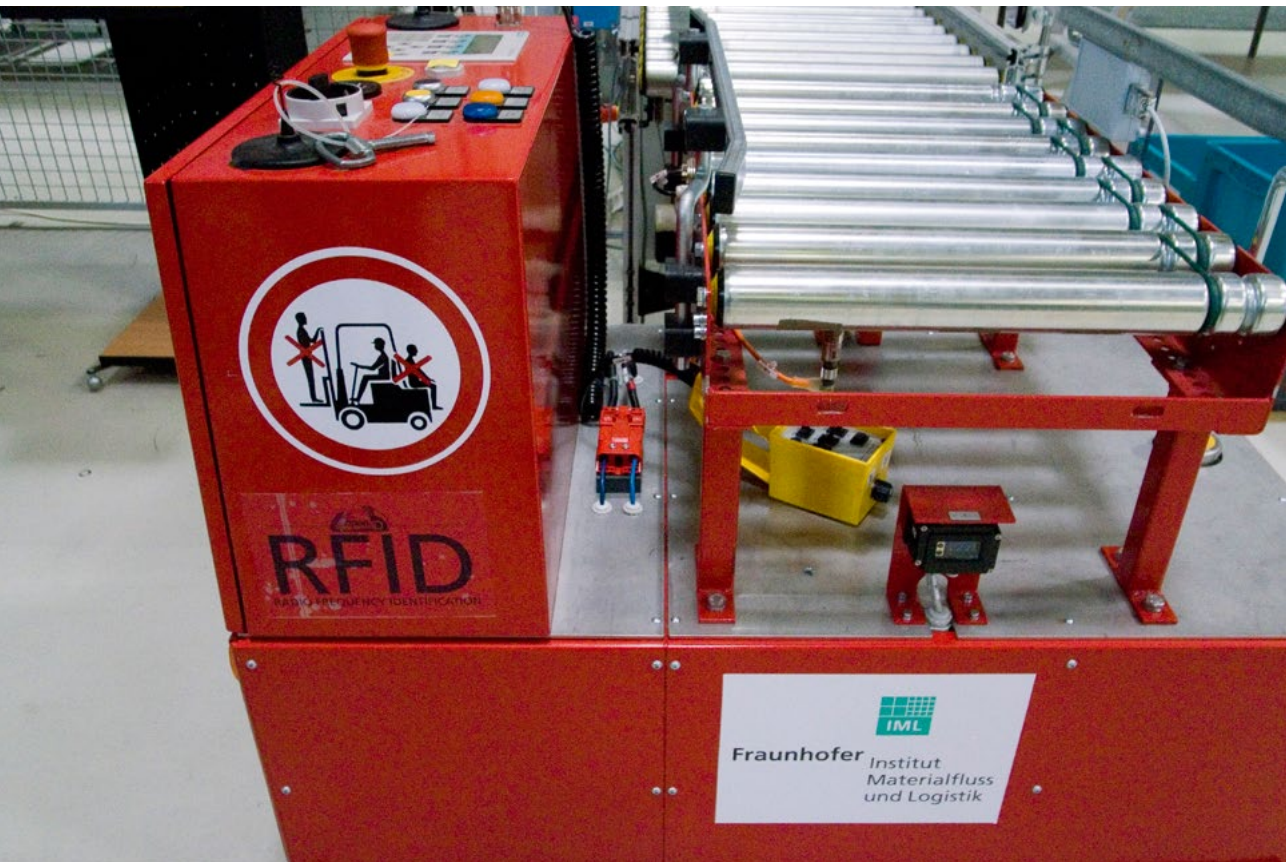
Figure 15: RFID systems in use in industrial logistics systems, where a reader is placed to identify objects passing by on a conveyor. Image from the author’s visit to the Fraunhofer Institute for Material Flow and Logistics (IML) in Dortmund, Germany.
