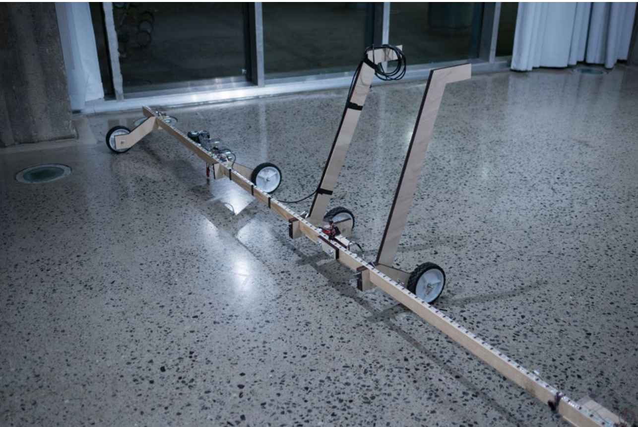
Figure 51: The 'GPS heat map' rig, designed to draw the signal strength of GPS signals as a giant light-painting across the ground.
