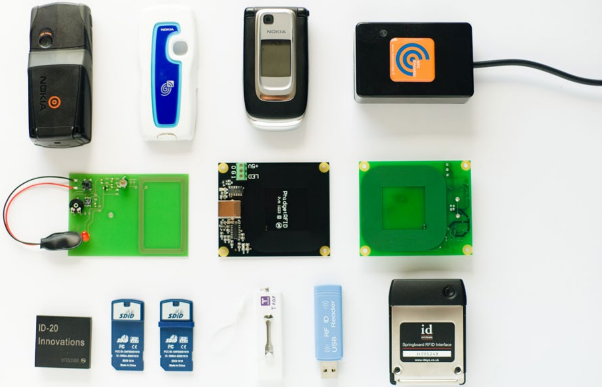
Figure 13: A collection of RFID readers, showing that readers can be embedded inside many different kinds of powered devices, including mobile phones, SD cards and USB dongles.
