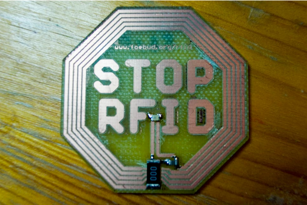
Figure 17: An “RFID detector” in the shape of a stop sign, designed and sold by FoeBuD. This simple circuit will make a light blink when in the presence of RFID radio signals, alerting the owner to potential privacy-invading electronic snooping.
