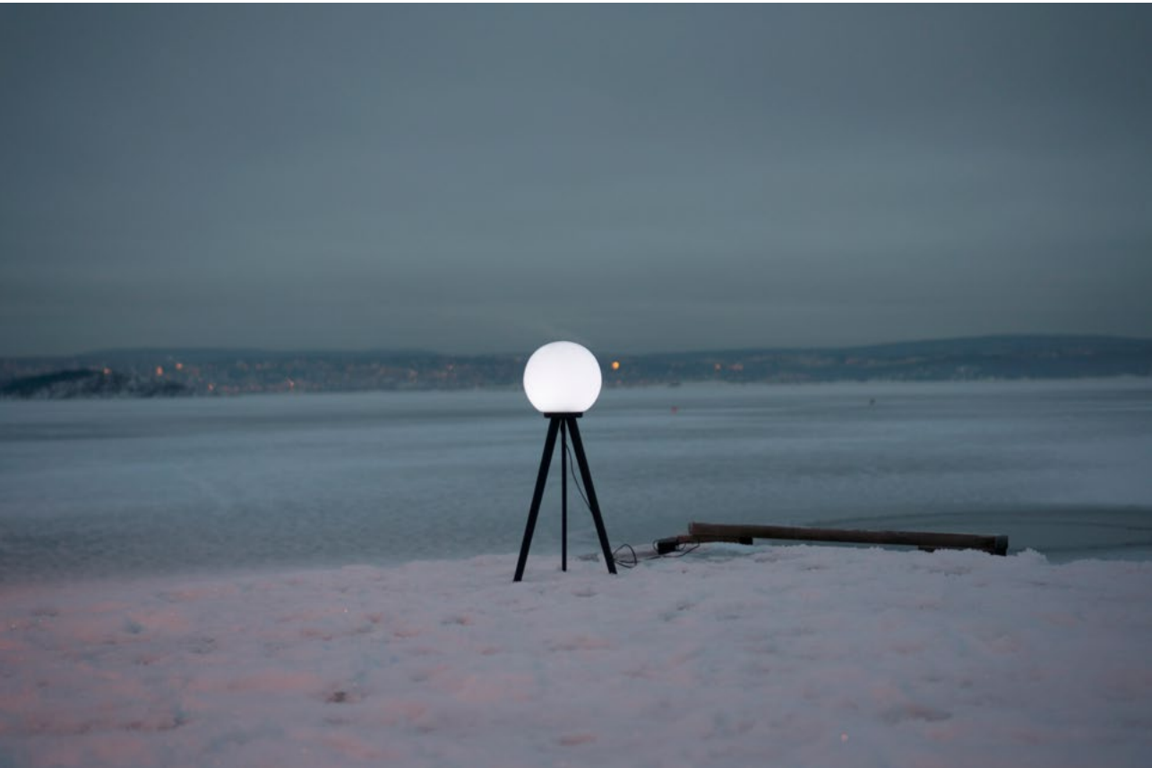
Figure 53: The final design of a 'Satellite Lamp'. This lamp changes brightness according to the accuracy of the GPS signals it detects. When we film it over many hours, as a time-lapse, we get mappings of GPS signals over time.
