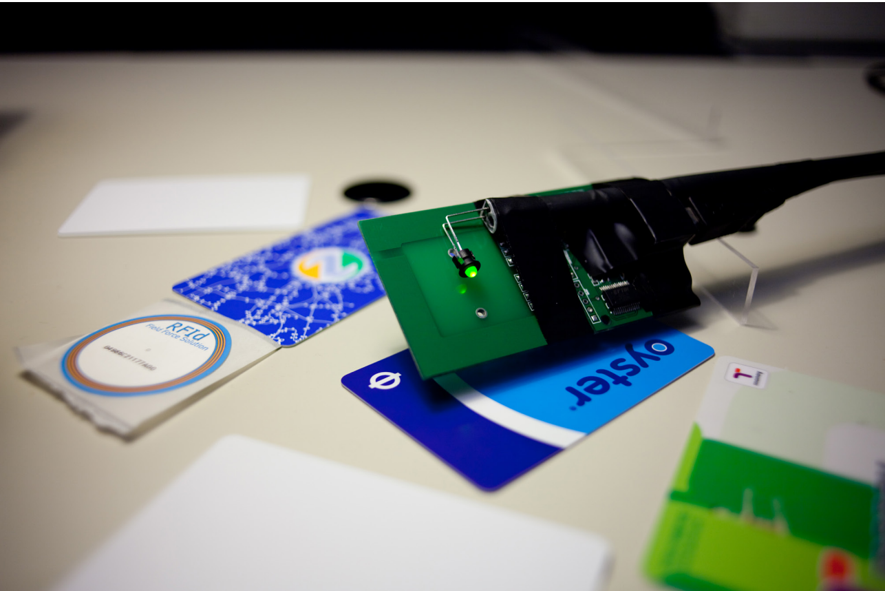
Figure 3.6. One of several versions of the RFID probes developed for creating the visualisations. This probe used a SonMicro RFID reader to detect the presence of an RFID tag. A piece of custom software turned this detection signal into a short flash of an LED.
