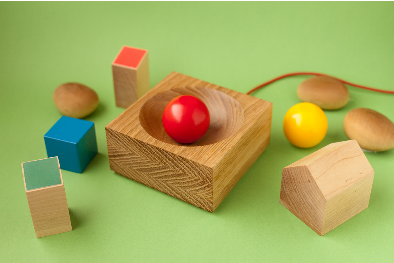
Figure 3.3. Skål is a token-based media player for children, where RFID tags embedded in toys are used to control media content, such as films and pictures. With this product we wanted to re-imagine RFID aesthetically and contextually, thus getting away from utilitarian, industrial applications and moving towards playful, domestic settings emphasising materials, colours, and interactions ( http://www.skaal.no ).
