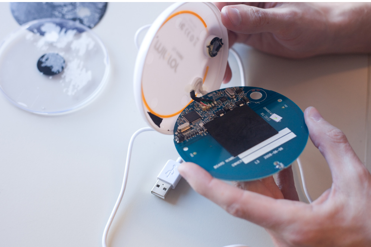
Figure 3.32. Reviewing interactive products involves not only analysing their interactions and product design, but also examining their technical solutions. This often involves dismantling products, such as the ‘Violet Mir:ror’ networked RFID reader, shown here. Credit: Timo Arnall.
