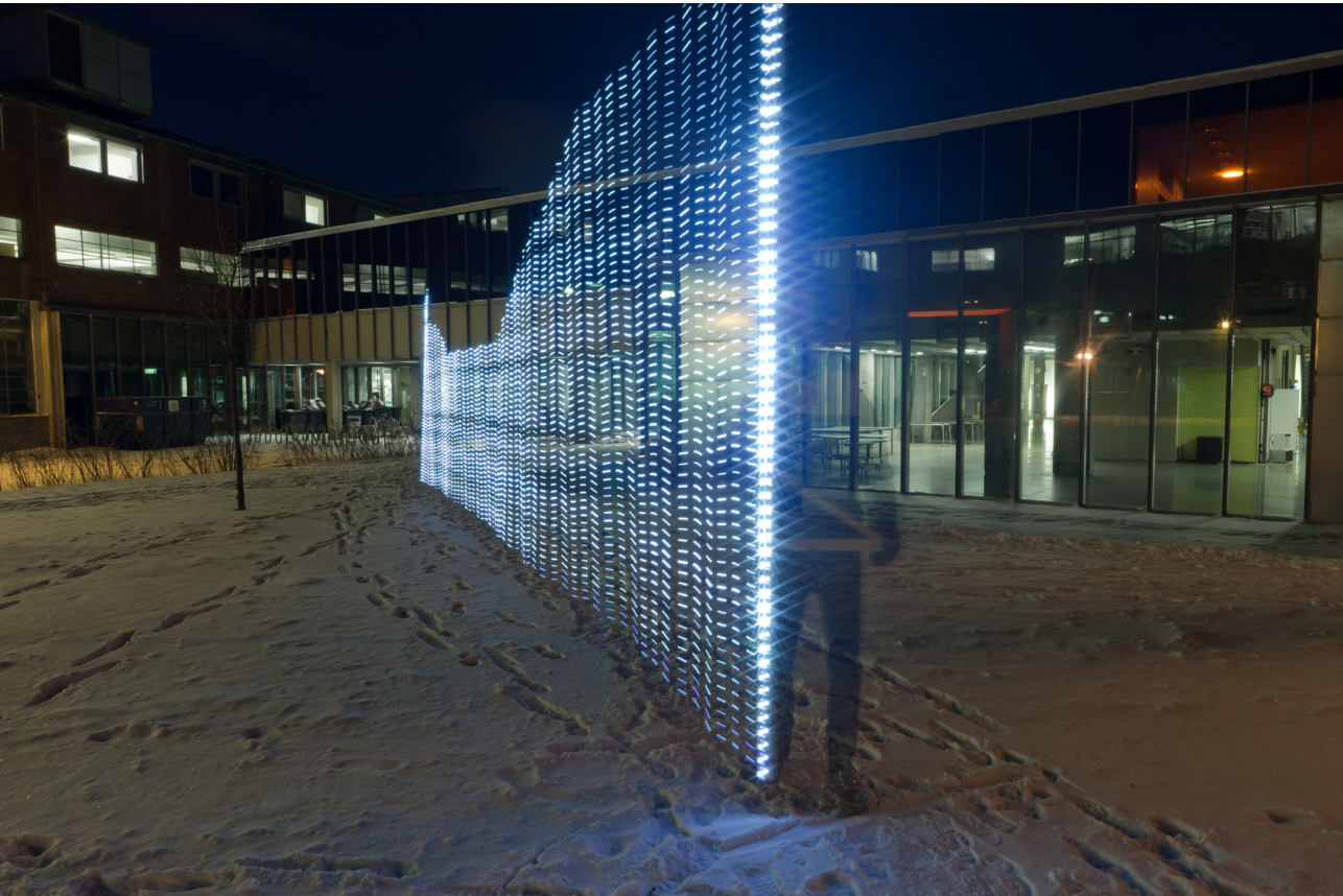
Figure 3.7. In this still from Immaterials: Light Painting WiFi we see the WiFi measuring rod being used. The rod consists of a four-metre-high column of LED lights and a WiFi receiver. The height of the light column is controlled by the strength of a chosen WiFi network. When the rod is moved through space and photographed using long exposure times, it draws a cross-section of the signal strength of the network.
