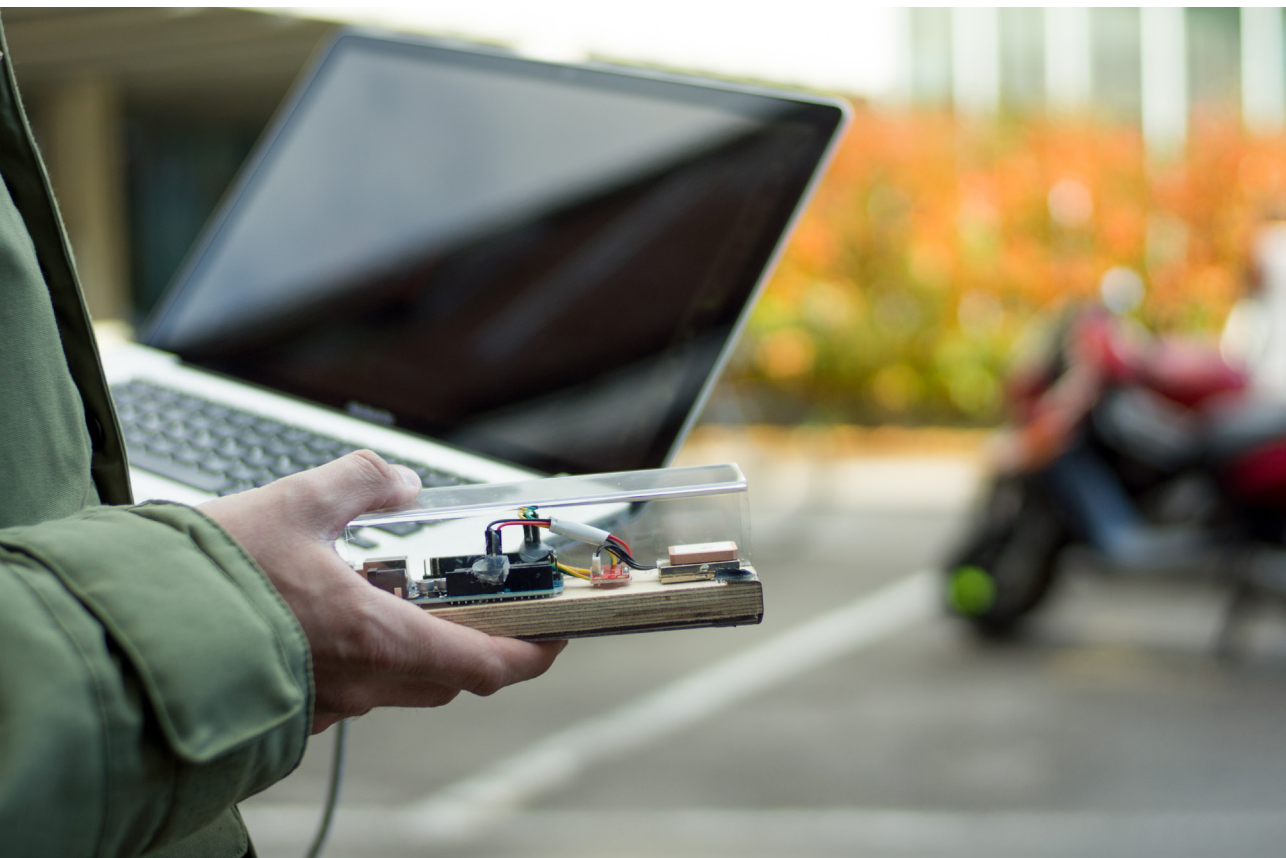
Figure 3.38. This is a GPS probe built specifically for logging and graphing changes in different GPS variables in the field. The probe communicates with a custom piece of software that graphs out variables in real-time.
