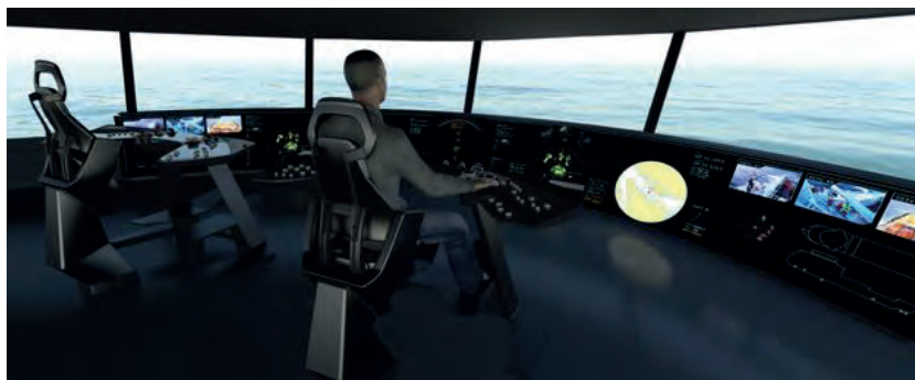
Figure 1. Picture of a future ship bridge produced in the Ulstein Bridge Concept research project. The bridge concept shows how focus on the interaction between user, ship and operation is materialised through new concepts on interaction and technology. The concept also brings in a new mind-set on the bridge, which must be seen as a holistic interface and not as separate modules as is the case on most ship bridges today.
