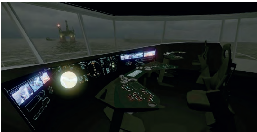
Figure 34. Screenshot from a game engine of the Ulstein Bridge Vision concept from the bridge at night. A first person perspective is used in avatar mode to get an impression of how the scenario can be experienced by a user to discuss how the bridge should be used at nighttime.
