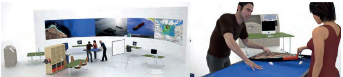
Figure 3, The picture show an oil-spill scenario simulation where information is placed on the multi-projection wall and a tabletop is used to combine physical representation with digital representations.
