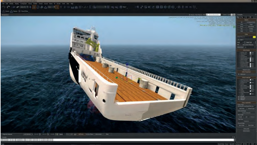
Figure 5. Screen capture of a physics simulation of cargo handling on a platform supply vessel. The barrels on deck represents heavy steal cylinders. While the simulation is running, it is possible to move them around on deck to change the load condition. This will affect the ship stability.
