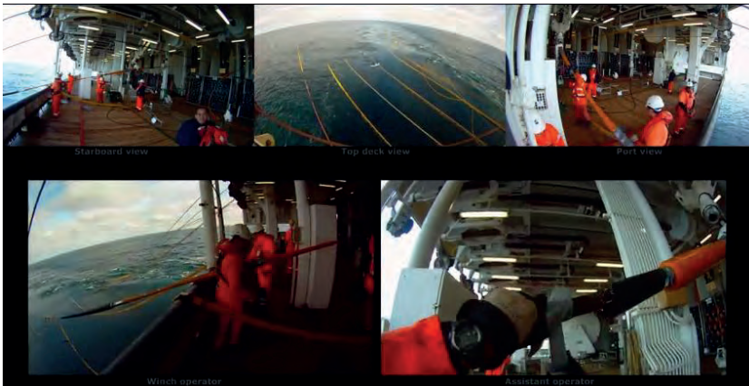
Figure 17. Video capture of the seismic recovery operation with multiple view angles showing the overall operation view and tasks performed by crew and winch operators this method gives a micro and macro perspective of the operation. Five camera angles are used and synchronised simultaneously.
