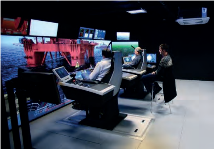
Figure 14. An anchor handling vessel simulator shows how complex scenarios can be simulated and used as a training facility and for the assessment of dynamic positioning operators. This is an anchor handling operation that requires very precise manoeuvring keeping attention to engine load, anchor angle to the rig, deck and ring communication. (Photo: Kongsberg Simulation)
