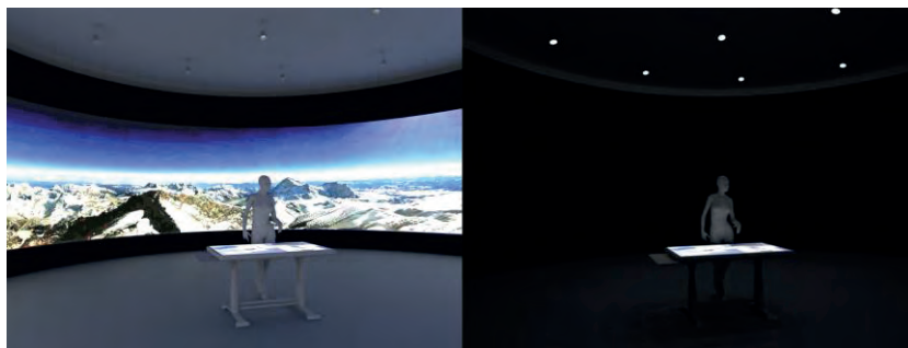
Figure 12. Screen capture from the SimSam-lab light simulation mixing multiple light sources. The room was modelled based on the architect drawings of the room. The light coeerce in the sealing was based on the IES light diagram from the manufacturer.
