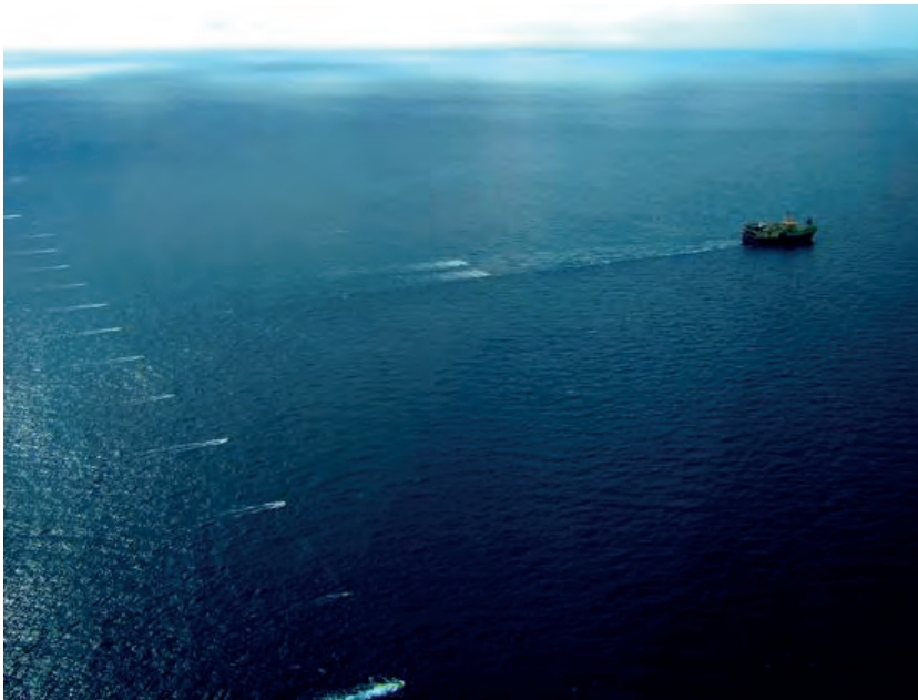
Figure 13. Picture from the Ramform Vanguard seismic ship with all 16 streamers deployed. The seismic streamers are stretched out 1.5km using hydrodynamic doors on each side of the streamer configuration. When all are deployed the length can be up to 8km. This makes the streamer operation cover an area of 12\text{km}^2 with a speed of 5knot making it the largest moving object in the world. (Photo: PGS)
