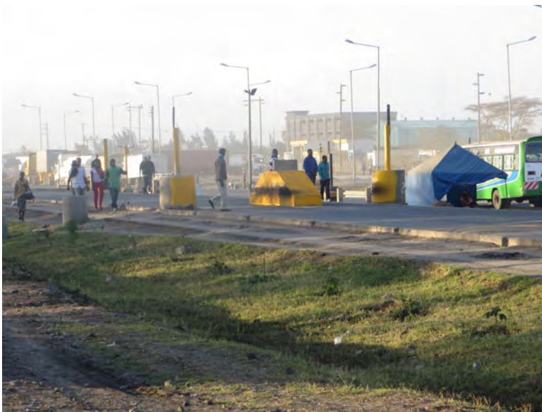
Plate 5.31: A picture of makeshift road barricades erected by Kenya Revenue Authority, the Kenya Police and the County Government of Machakos at Mlolongo along the Mombasa Highway after the transformations. Such barricades are used to constrain the movements of sand trucks to prevent them from evading the weighbridge. The dark streaks on the barricades indicate that vehicles scrape and are scraped by the barricades. (Source: Author)
