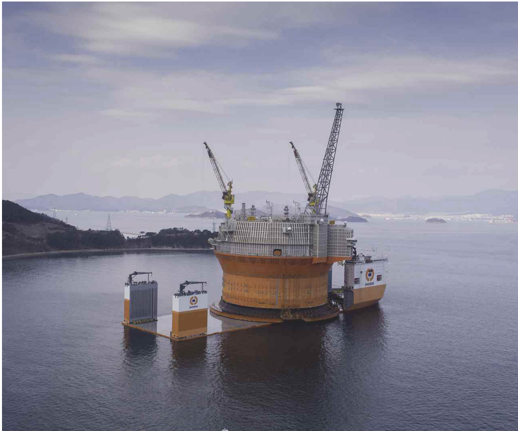
Sevan 1000 FPSO being towed towards the Goliat site on board the Dockwise Vanguard
