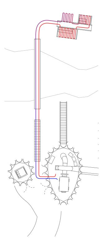
Excess heat transfered to sauna, through waterborne heating.
