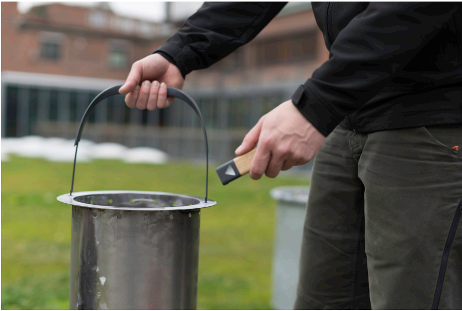
Detach the magnetic control stick to safely tilt and empty the biochar content
