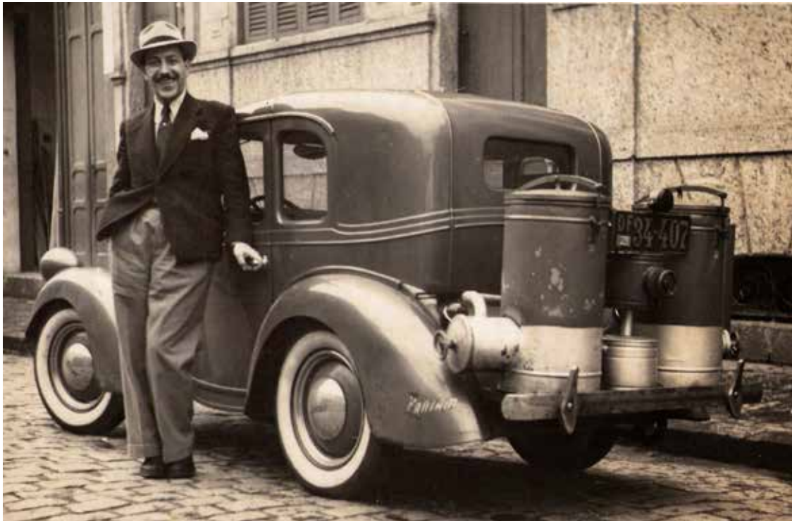
Car with syngas reactor. (Gomes, 2011)
