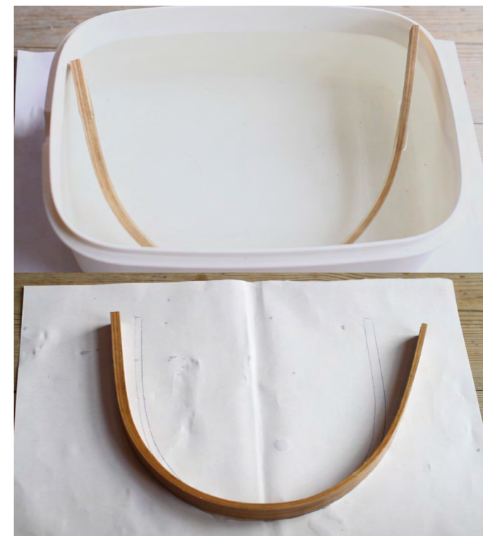
An U bend soaked in water, to study the movement when exposed to moisture
