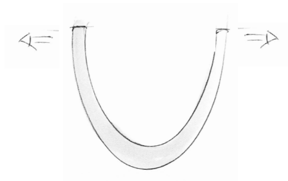
Movement of an U bend, when exposed to moisture
