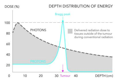
Diagram showing the bragg peak making it possible to control the distribution of energy with protons.
