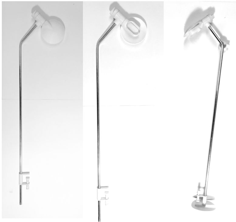
Small scaled model are made for shape testing, the proportion is 0.4:1
