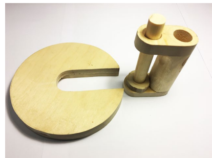
The size of the base is 200mm diameter, I tried 300 diameter as the floor lamp version. The base is too big, too dominant, so that in the end the dimension of the base is 200mm*20mm, if it made in steel it can offer more than 5kg weight, which is enough for the floor lamp.
