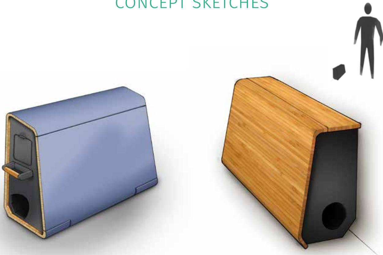
These concept drawing are quite close to what I ended up with in the end. Although at the time I was considering creating a core out of ABS and the outer shell in laminated wood.
