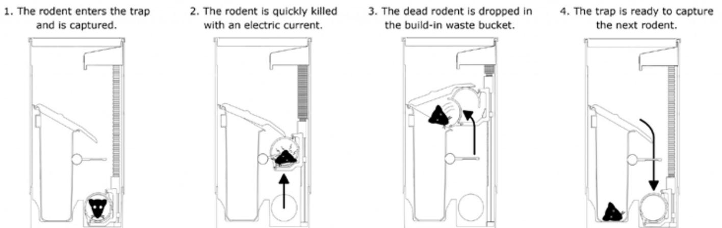
The inner workings of the Smart Box. The trap has prongs which the rat is hoisted up into ensuring that the electric current goes through the head causing swift loss of consciousness. The trap can hold 5-7 rats before it has to be emptied by a technician
