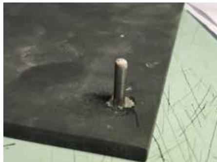
Steel pegs were attached to the front cover. These will lock into place by magnets inside the end pieces.
