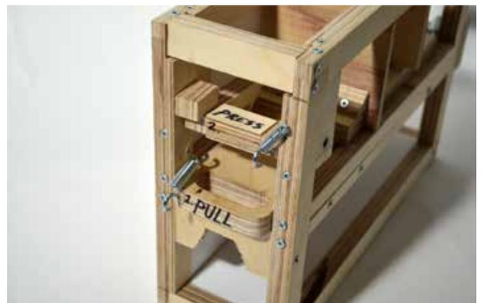
The mechanical model is a bit overengineered and bulky compared to the final product but it works well as proof of concept. It is made out of plywood, foamcore and a whole lot of screws.
