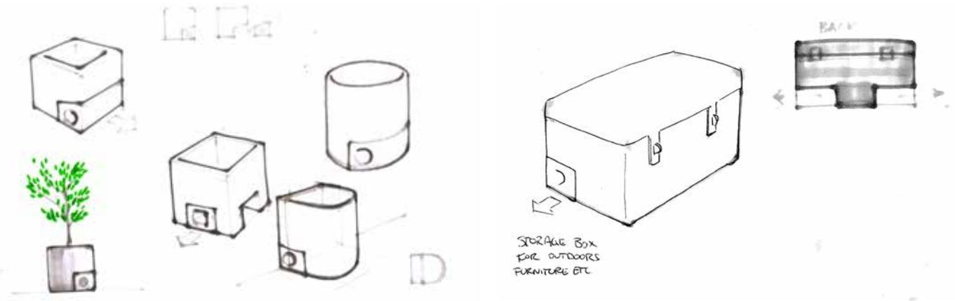
Early in the project there emerged a concept that was about concealing and camouflaging the trap in different objects such as an outdoors planter or an outdoors storage box. This concept had potential for a user desiring a more discreet trap.
