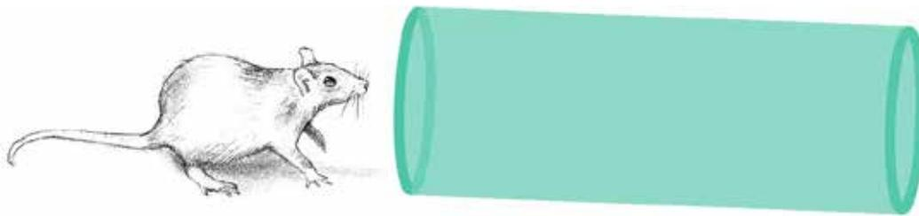
A rat might hesitate to enter a trap if it is perceived as a dead end. If we shape it like a tunnel the rat will probably feel more at ease and we will have greater success at luring the rat into the trap. The tunnel shape also means twice as many entrances.
