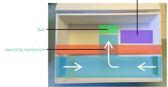
Basic schematics of the layout. The blue shows the t-shaped tunnel with two openings and the bait enclosed in the middle. The trap springs when the rat pokes it head up towards the bait.
