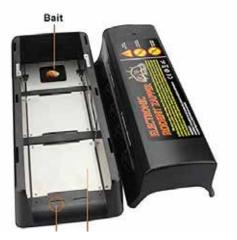
Here we see a rat trap called *Hoont* with the top lid removed. Inside we see two metal plates which will electrocute the rat when it steps on both at the same time
