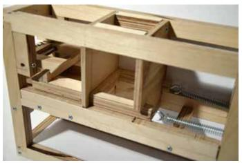
To the right we can see the springs which pulls the bar shut. They are attached in the opposite end from the handle.
