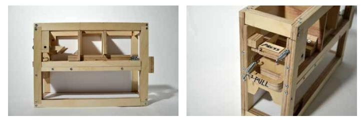
The mechanical model is a bit overengineered and bulky compared to the final product but it works well as proof of concept. It is made out of plywood, foamcore and a whole lot of screws.
