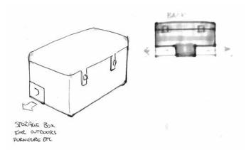
Early in the project there emerged a concept that was about concealing and camouflaing the trap in different objects such as an outdoors planter or an outdoors storage box. This concept had potential for a user desiring a more discreet trap. But in the end I decided to focus on designing a more aestethically pleasing trap so that perhaps the user wouldn't see the need for hiding the trap away.
