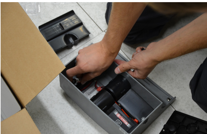
A technician putting batteries into a new I-trap
