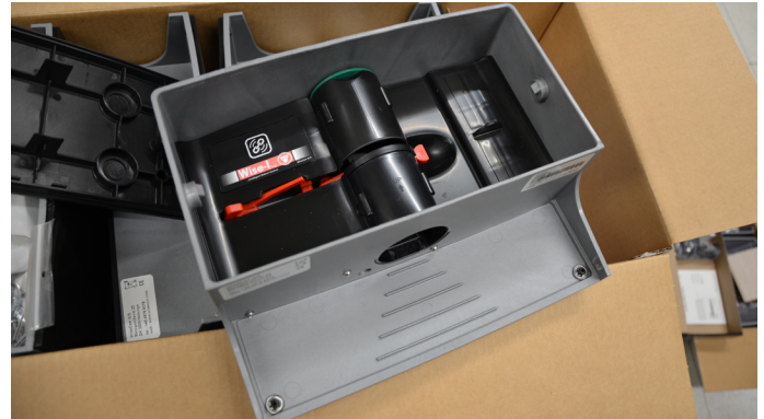
The backside of the Wisecon I-trap. Here we can see a small tube which has bait at the top. The rat will poke its head in from below getting hit in the neck by the red spring loaded swing arm.
