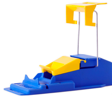
Mjölner rat trap. Compared to the classic trap this does a better job at guiding the rat into the correct position. The yellow hatch in the middle contains the bait. The rat will try to poke it open with its nose and springing the trap in doing so.
