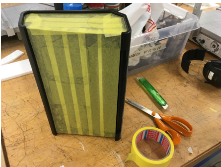
Masking of the model before applying the second color.
