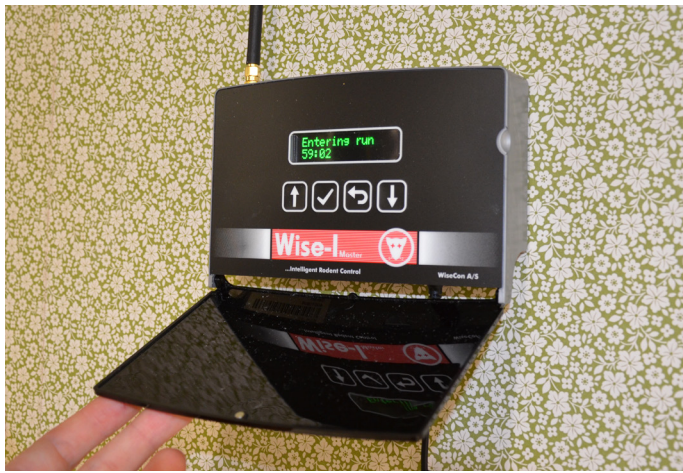
Master unit up and running. Ready to report activity over the cellular network.
