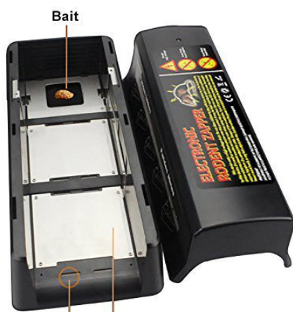
Here we see a rat trap called Hoot with the top lid removed. Inside we see two metal plates which will electrocute the rat when it steps on both at the same time
