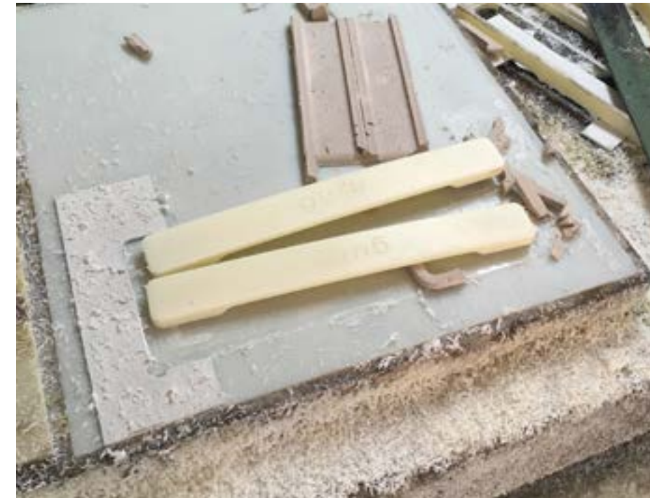
I contacted a CNC model factory in Shenzhen, and build the prototype in ABS .
