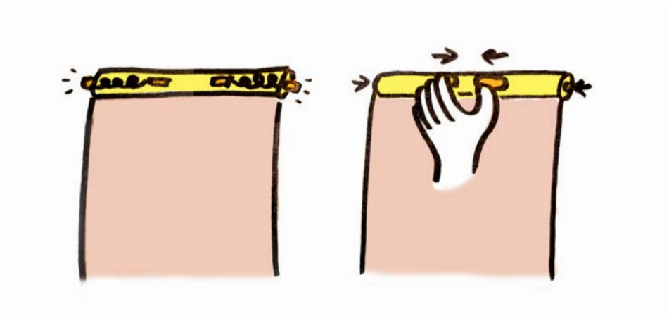
The rolling handle has two telescopic feet, which can be controlled by the user.
