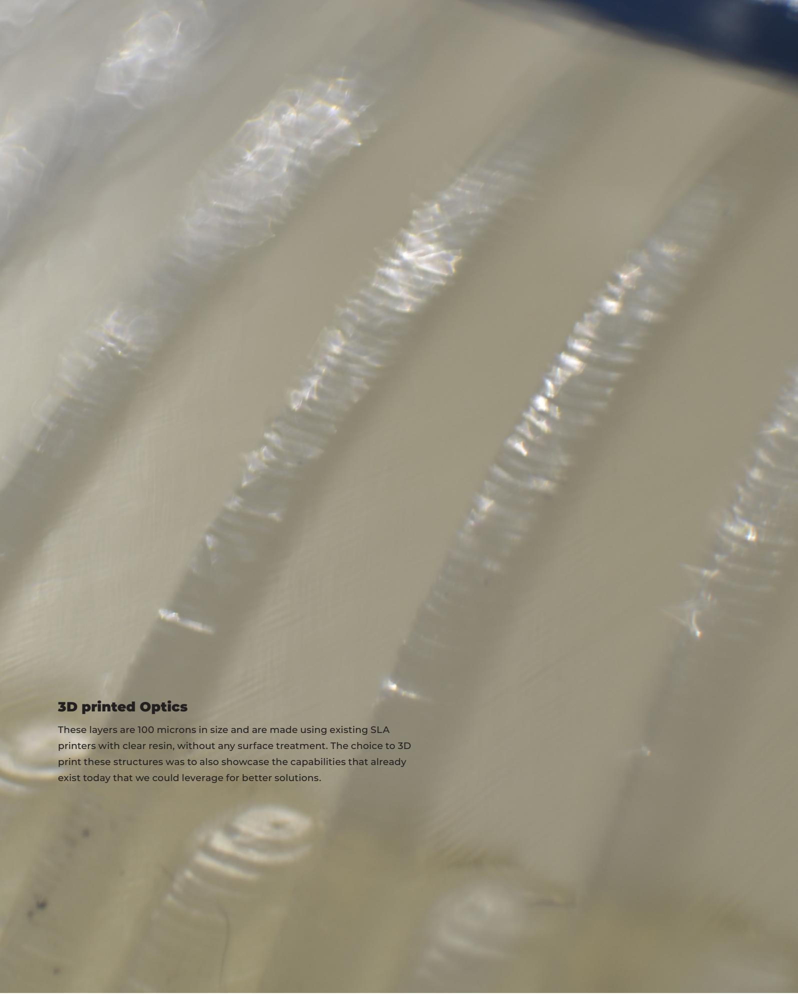
A close-up photograph of several parallel, cylindrical optical structures printed in clear resin. The structures are arranged diagonally across the frame. Each structure has a series of fine, concentric ridges or grooves around its circumference, creating a textured surface. The lighting is soft and directional, highlighting the intricate details of the printing process and the transparency of the resin. The background is a plain, light-colored surface.
