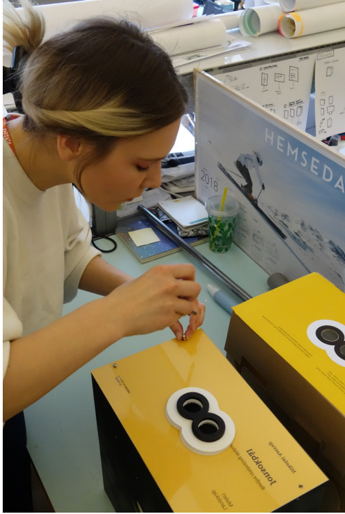
MAKING THE PROTOTYPE A wooden housing for the screens that needed to be dark inside, easy to open and solid. Also a concrete stand to counterweigh the top heavy box.
