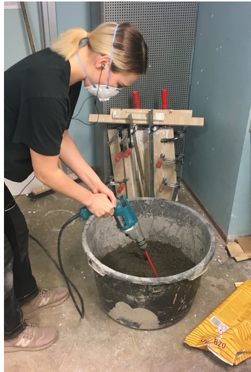
MAKING THE PROTOTYPE A wooden housing for the screens that needed to be dark inside, easy to open and solid. Also a concrete stand to counterweigh the top heavy box.
