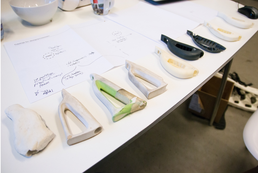
Figure 24 - A timeline mapping of the development of an ergonomic ski-pole grip. Photo: William Kempton.
