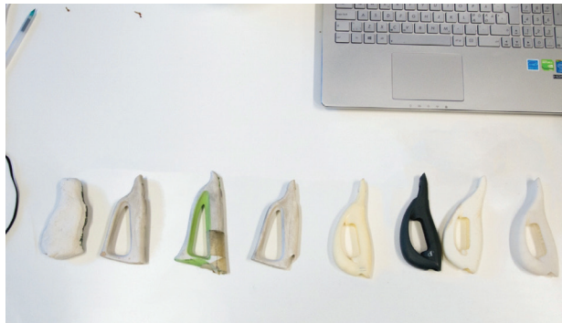
Figure 4.12 Incremental development (left to right) through a series of models from the DF1 ski pole grip. Photo: Pivot Design.
