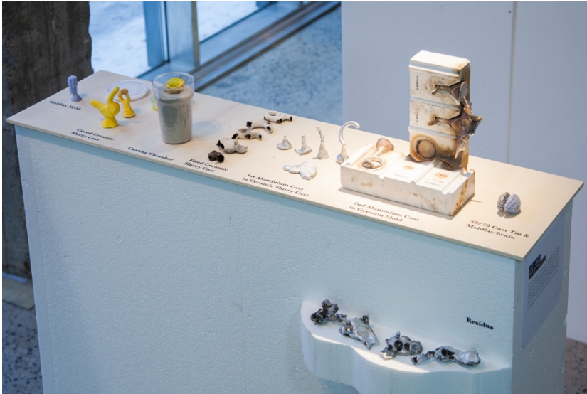
Figure 18 – Students’ attempts at making aluminium casts using both FDM-based and 3DP processes. Photo: William Kempton.
