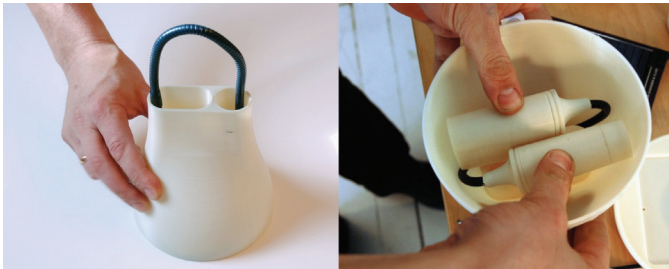
Figure 4.7 Initial negotiation of usability, functionality, and shape with initial rapid prototypes made with the in-house FDM 3D printer. Photo: K8.
