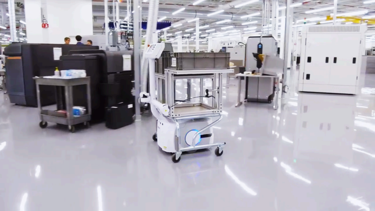
Figure 31 – A mobile robot transporting trays of 3D printed components at Ford's recent Advanced Manufacturing Centre in Glendale, MI. The $45-million centre, which is seen in this caption in a promotional video, is advertised by Ford as the 'reinventing' the assembly line, which is significant to Ford's manufacturing heritage (Ford Motor Company, 2018). Photo: Ford Motor Company.
