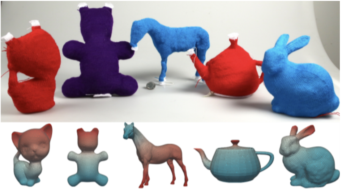
Figure 3.5. 3D models (bottom) and the knit models created based on them (top). Note that the rabbit is stuffed with a foam model to give it its precise shape.
