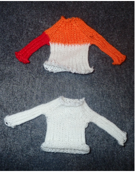
Figure 9.2. Top: first iteration miniature shirt made with three yarn carriers. Bottom: second iteration shirt made with one yarn carrier and improved technique for joining sleeves.
