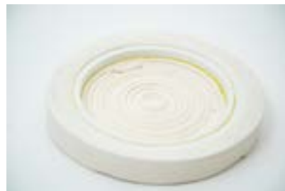
Damaged the plaster surface during demolding
