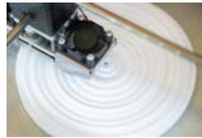
Print out positive for mold making
