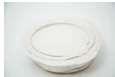
Damaged the plaster surface during demolding
