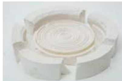
Leaving air bubbles on the surface after demolding
