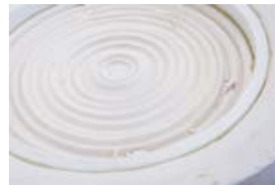
Damaged the plaster surface during demolding
