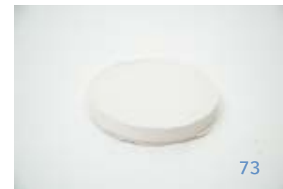
Silicon second Cast, with a release agent, pretreat
