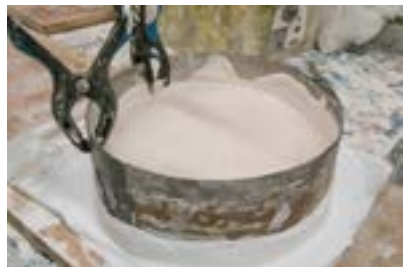
Plaster A: Drying too fast
