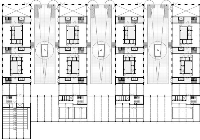
The bicycle garage and storage rooms run through the basement plan of the building connecting the north side of the complex to the south side. This allows all the residents to reach the car garage or the bicycles and to exit the complex in all directions based by foot or by wheel.
