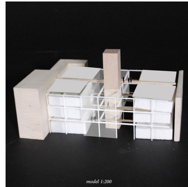
Study 8; central atrium with bridges Cutting holes in existing slabs.
