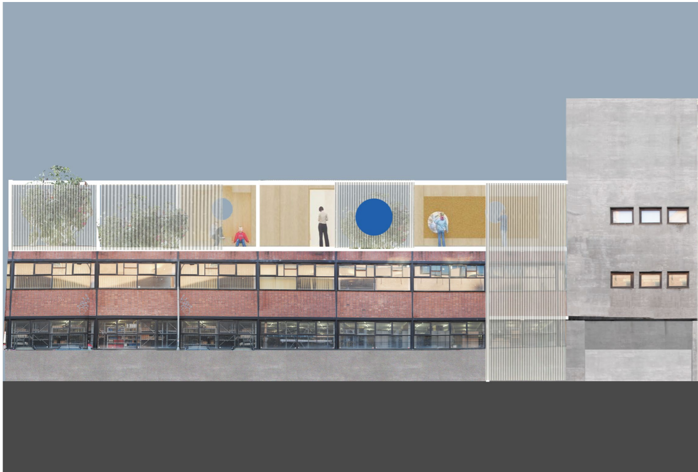
Steel frames, replacing existing facade
