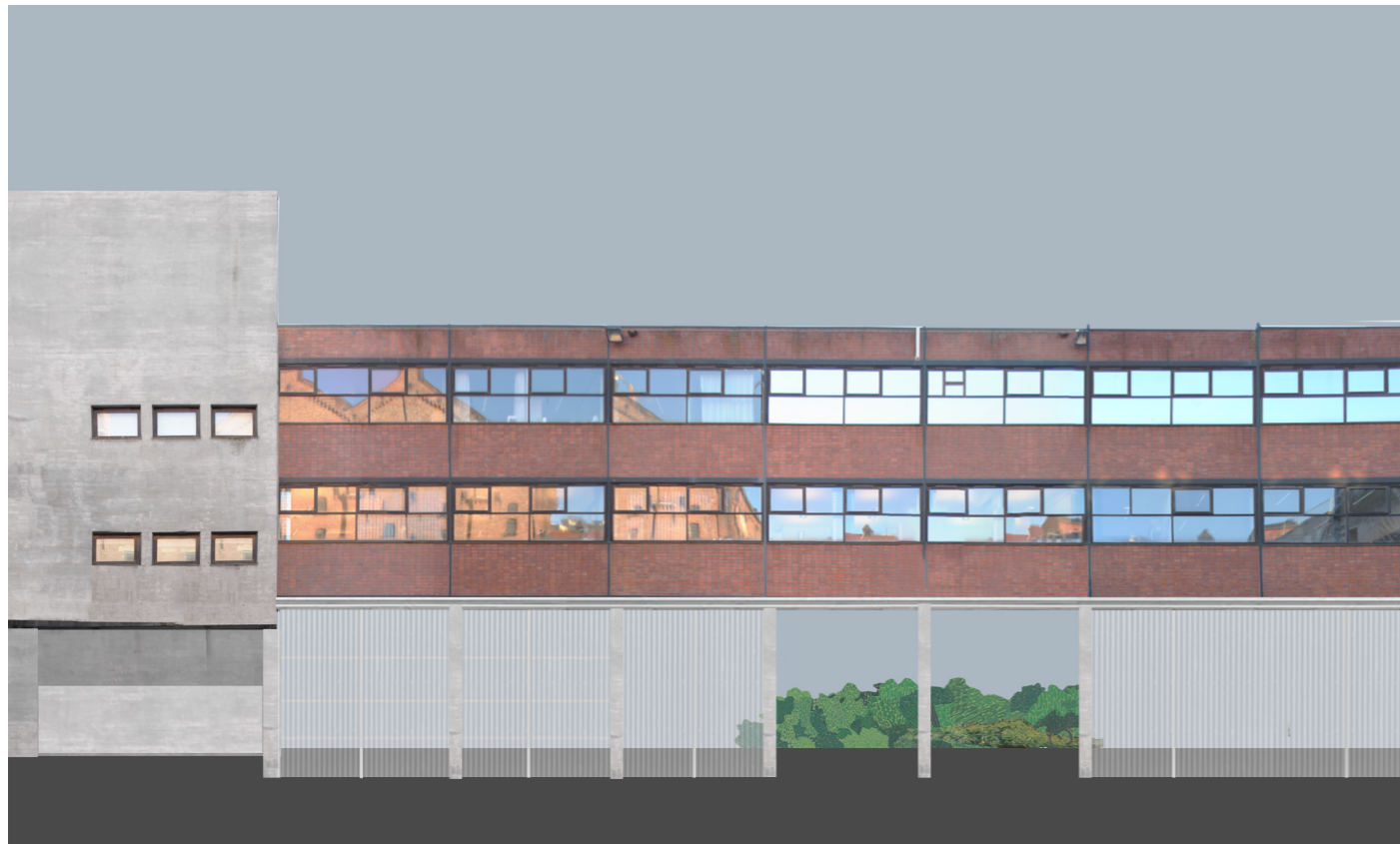
Static polycarbonate facade
