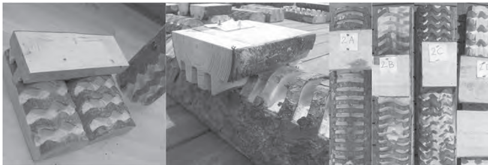
Figure 4 The BackToBack wet-in-wet concept. Tests of various incision patterns.
