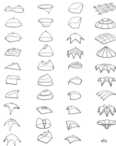
Figure 106 Heinz Isler, 1959, 39 possible shell forms and "etc".
