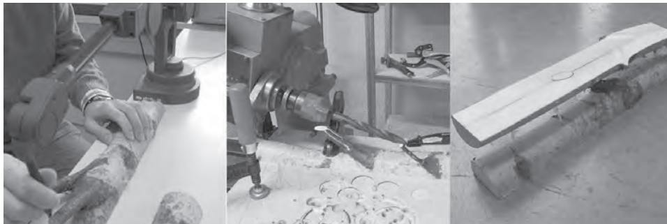
Figure 5 Stumps-in-boles. From 3D scan to tiltable drill press and assembly
