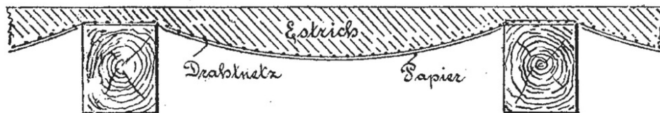
Figure 97 Gustav Lilienthal, 1898, Terrast Decke , a fireproof ceiling made with wire netting, paper or fabric, and screed.
