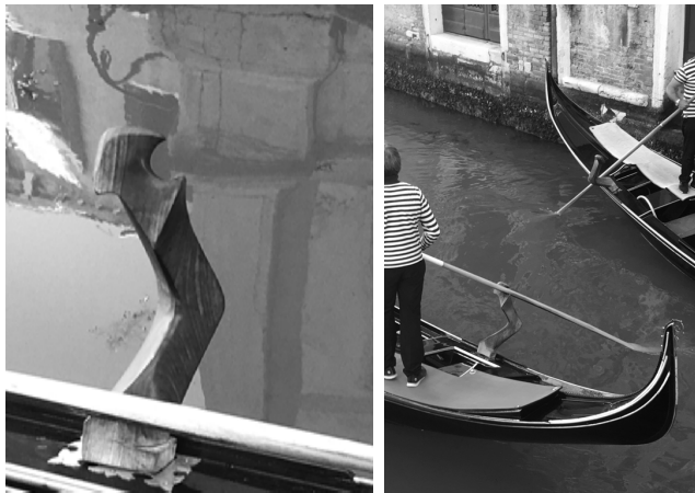
Figure 91 Fórcole . Left: The complex shape. Right: In use with an oar.
