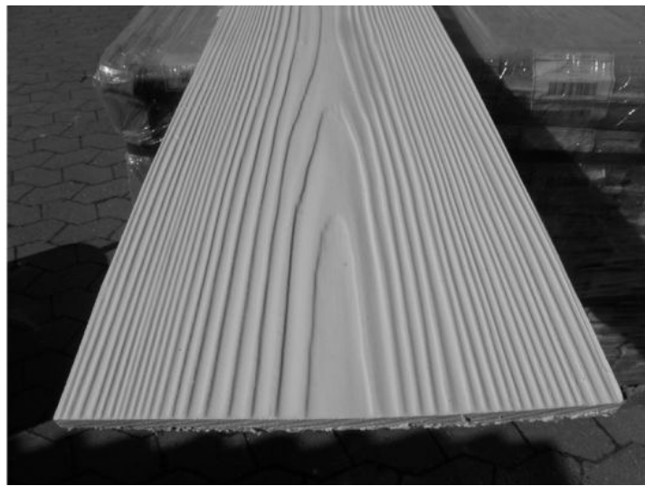
Figure 78 Skeuomorphism: fibre-cement panel imitating wood grain.
