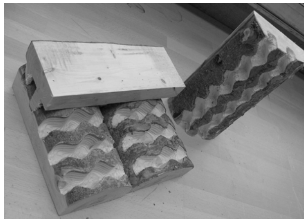
Figure 30 BackToBack , wet-in-wet system.
