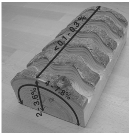
Figure 29 Anisotropic shrinkage of Norway spruce.
