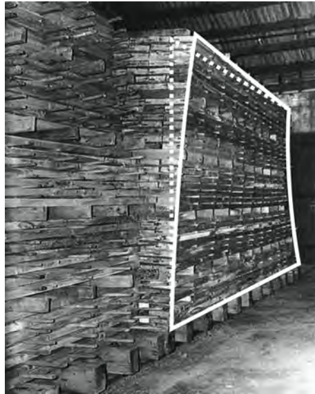
Figure 15 Twisted stack of timber after drying.
