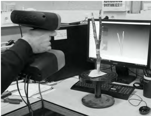
Figure 65 Y-timbers : 3D scanning.
