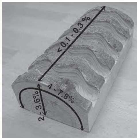
Figure 15. Orthotropic shrinkage in Norway spruce
