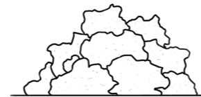
DROSS (x1) aluminium scrap burned once will create dross lumps
