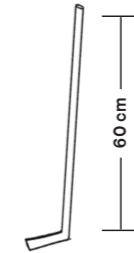
STEEL STIRER used to stir and mix dross and aluminium to create texture
