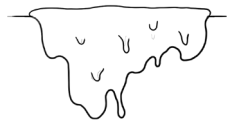
SUSPENDASLURRY (SUS) a paint like consistency, dip model to create a shell mold
