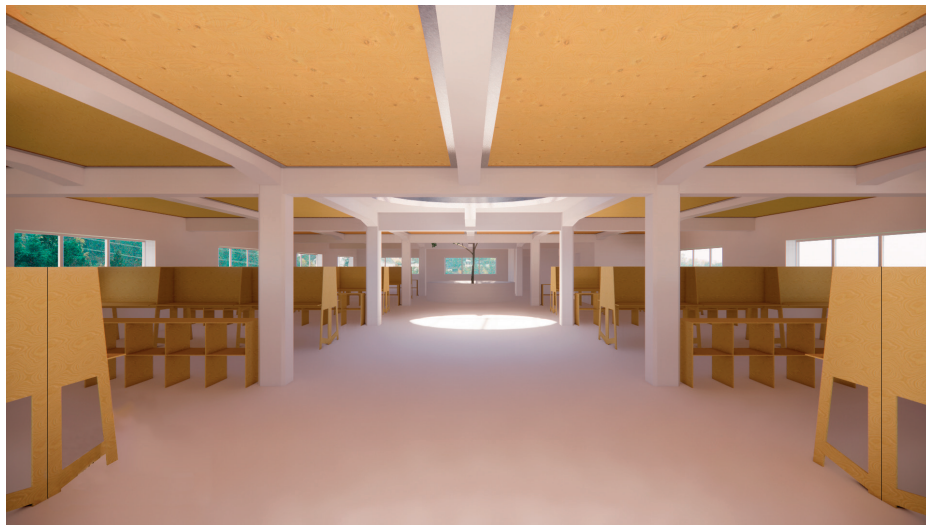
Loft: Highest floor. Illustration shows the new CLT ceiling and how it is hung between the original beams. Two holes are cut out in the original ceiling to enable light to enter the otherwise dark space.
