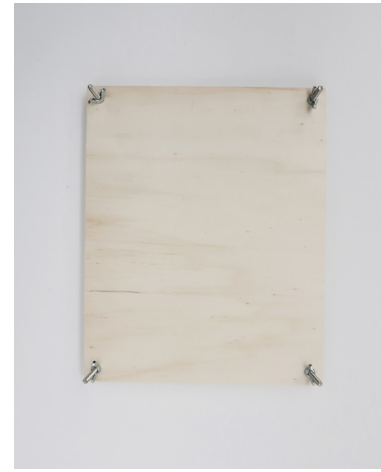
Plywood 5 mm 4 bolts 5mm 4 wing nuts 5mm 4 discs cardboard 1,5 mm
