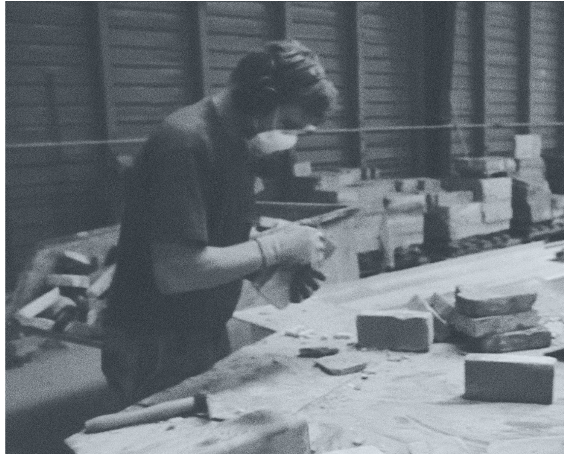
09. Processing of salvaged bricks at Gamle Mursten, Denmark. Salvaged materials are rarely ready for reuse. They often need to be processed, such as here where mortar is being removed from the individual bricks and quality checks are performed.
