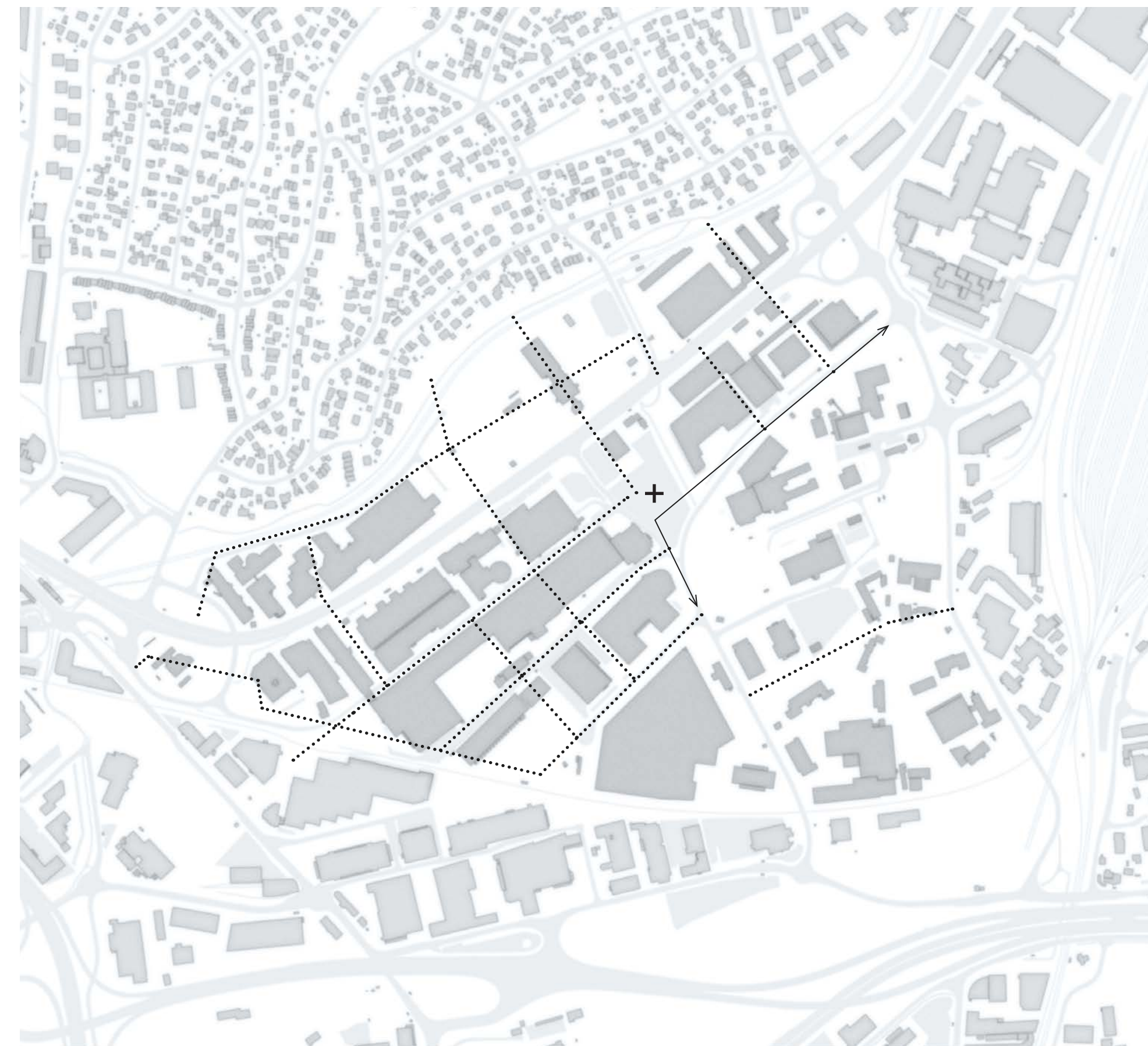
16. Future road network. The street Haraldrudveien, emphasized on the diagram, is to be straightened. On the corner of this new road, an area currently used for parking is to be turned into a city square. This diagram is a visual summary of planning proposals currently going through the application process, not proposals made by the author.
