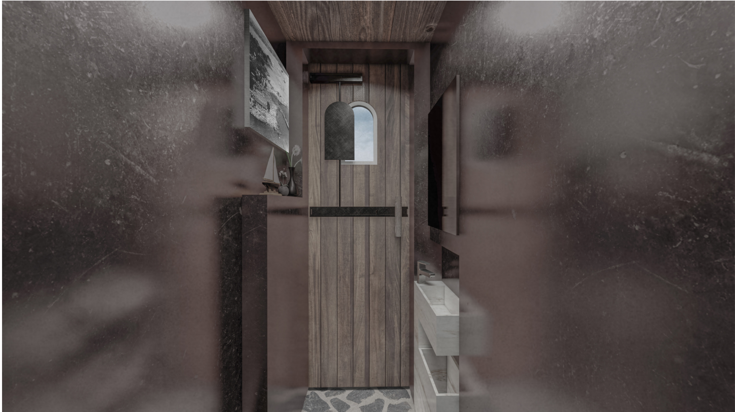
Interior of public toilets. Robust metal sheeting and slate flooring made for rough use. Lock mechanism provides shading for the window
