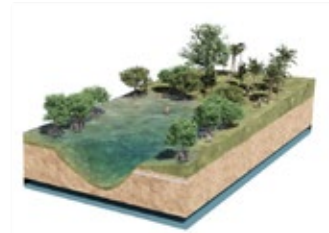
Wet pond, retention basin. Located in the course of a stream
