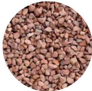
Crushed brick (recycled material)
