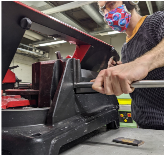
Cutting Pivot Pole to Size
