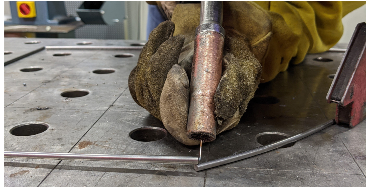
Tacking Frame Together
