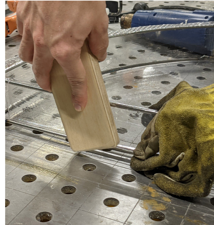
Forming Tray Around the Frame
