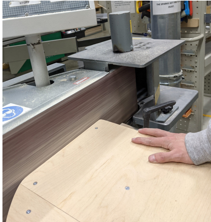
Sanding Mould Down to Size
