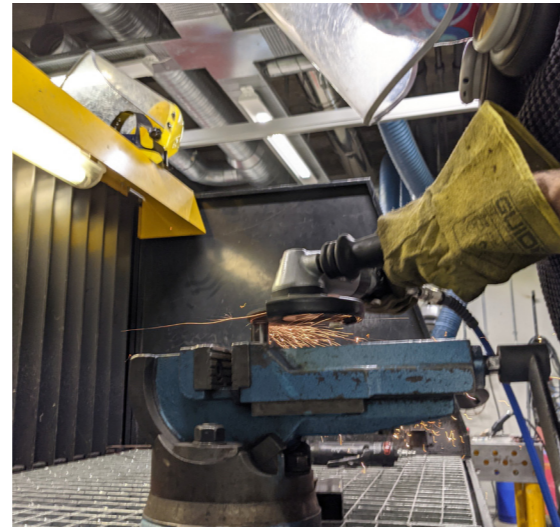
Grinding Shelf Supports
