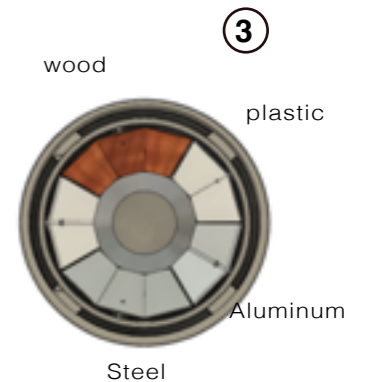
Sound panels with increased hardness, so they sharpness of their sound feedback increased.
