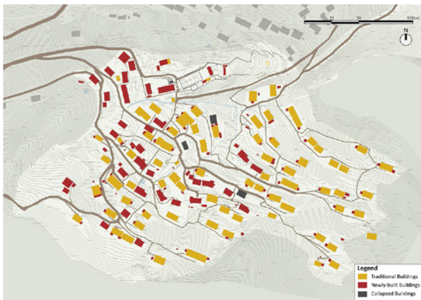
Figure 5.6: The diagram shows the situation before the renovation project started. The yellow-marked buildings refer to stilted architecture, the red-marked buildings refer to newly-constructed buildings built in the last decade, and the grey-marked buildings refer to collapsed buildings. (Source: Author)
