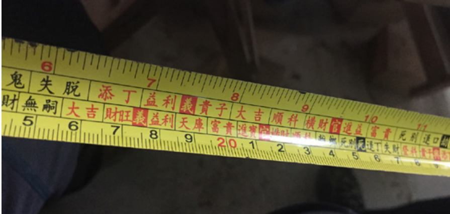
Figure 5.48: This Lu Ban chi (Lu Ban rule) used by craftsmen shows metric and British measurements and good and bad luck units. (Source: Author)
