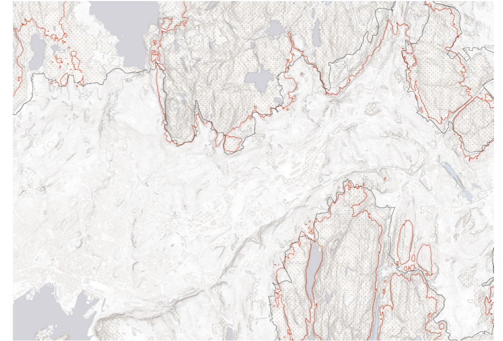
Contour 220: elevation until which drinking water could be supplied with natural pressure that gave the base for the first marka border. (Oslo Byleksikon)
