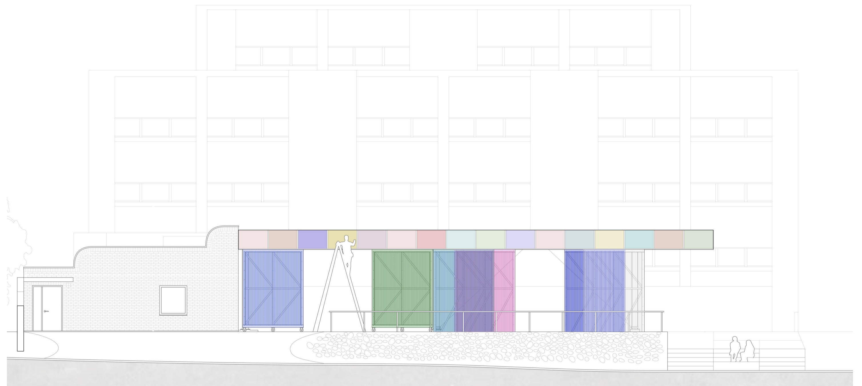
Western elevation 1:100. The canopy sides are clad with removable steel plate canvases, constantly renewing the site.
