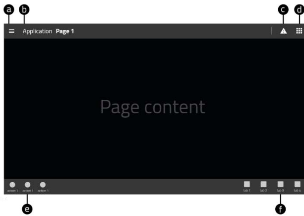
Figure 2: Main user interface window: a. hamburger menu, b. main title, c. alarm component, d. global navigation menu, e. action buttons and f. tab menu.
