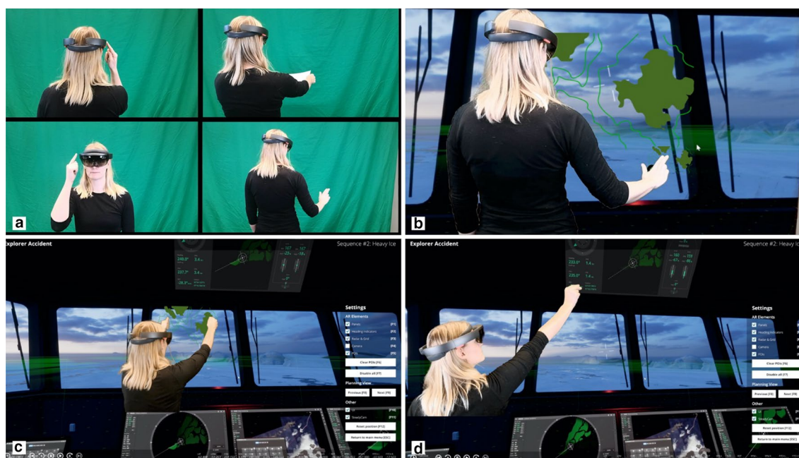
Fig. 5 A student group's testing of different forms of gestures for interacting with an AR map. a shows the use of greenscreen when filming gestures performed by one of the students. The greenscreen makes it easier to further process the recorded material. The recorded gestures were merged with recordings from the VRROS, alongside
