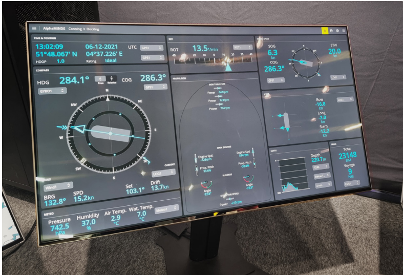
Figure 37: Application of OpenBridge Design System from the Industry Partner Alphasat JRC. (Photo: OICL)
