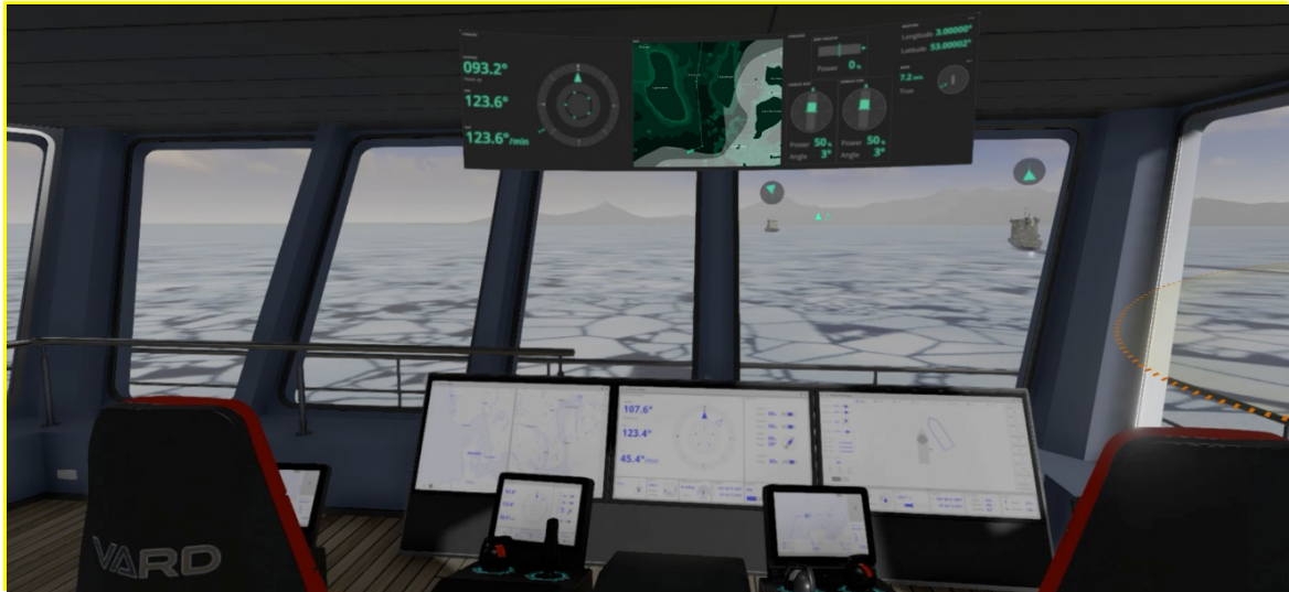
Figure 10. Screenshot from the mixed reality platform with prototypes of AR applications that follow the placement rules of the information areas: the sky band with apps, widgets and an AR map (top), the horizon band with annotations (middle) and the water's surface with an ocean overlay (right).
