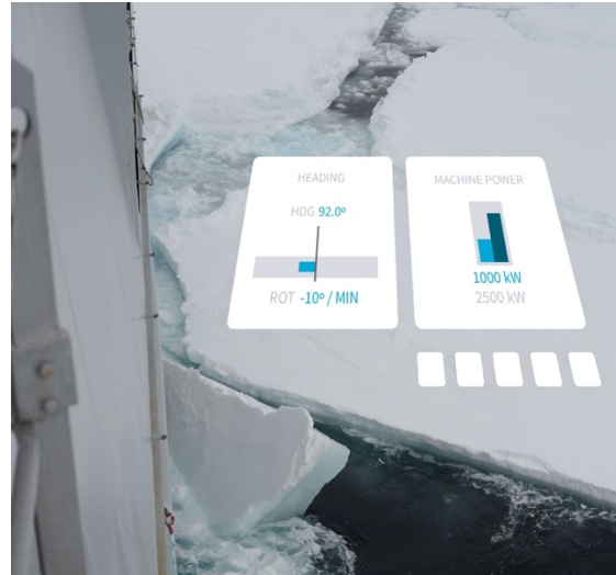
Figure 8: AR widgets representing selected information from the Conning system placed onto the ice.
