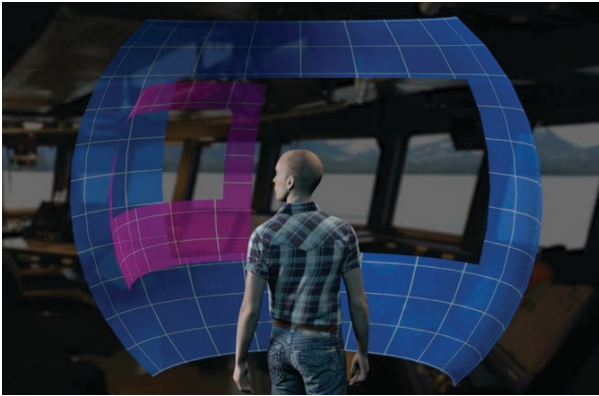
Figure 5: Representation of body spheres for fixing AR content divided into two categories: head-locked content and shoulder-locked content.
