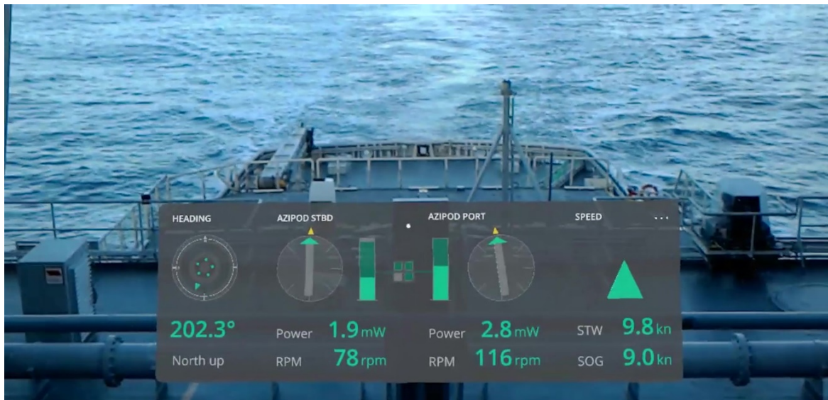
Figure 9. Free pinning of a container object with widgets attached to the back of the ship under the horizon band.
