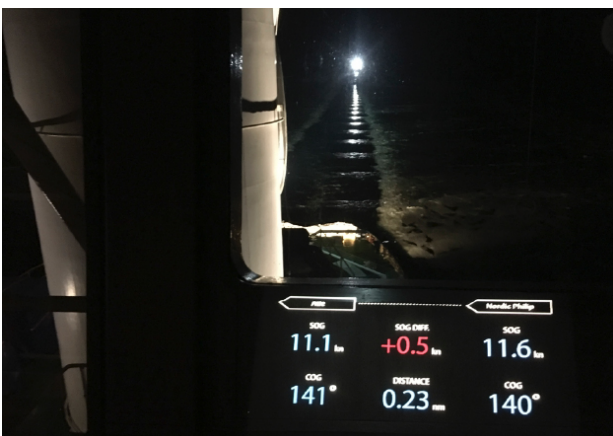
Figure 10: Design concept to indicate a ship's own relation to other ships by displaying information on a dark panel below the window. Prototyped by projecting graphics onto surfaces on the bridge using a portable mini-projector.
