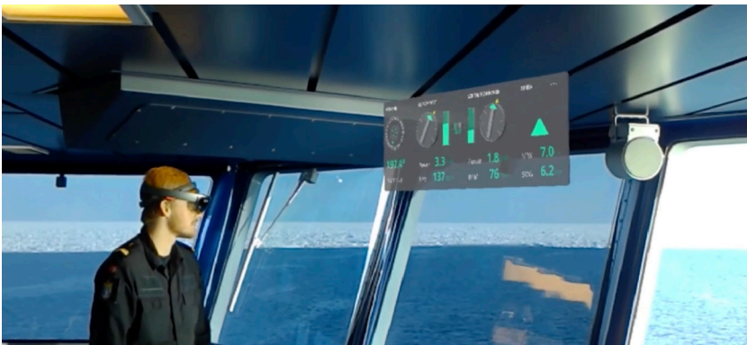
Figure 35: Illustration of how the navigator sees the digital UI components through HoloLens drawn and captured through HoloLens. (Photo: OICL)
