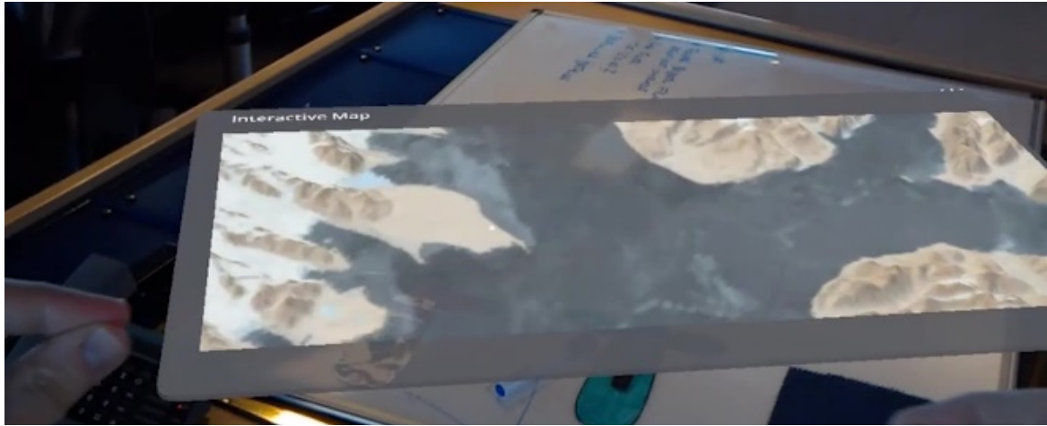
Figure 6. AR map concept of a map as a free object that can be placed anywhere, for example on a table used to plan a route through ice.
