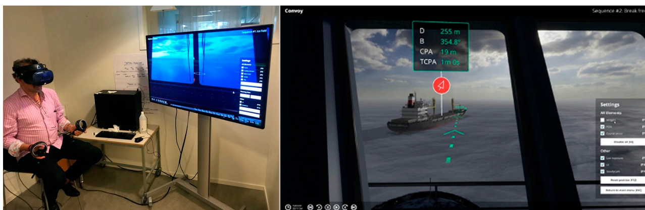
Figure 2. To the left: the setup of the virtual reality-reconstructed operation scenarios (VRROS) seen from an exocentric perspective which represents the test facilitators who can monitor both the user's behavior in the room and what the user sees in the VR headset on the big screen. To the right: a screenshot of representing the egocentric perspective of what the user sees within the VRROS.
