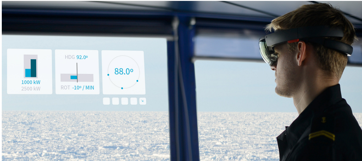
Figure 4: Illustration showing a design concept in which graphics are placed outside the window to accommodate the need to fix graphics to the environment instead of a body sphere (Photo: SEDNA).
