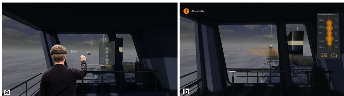
Fig. 4 Screenshots from a video in a student presentation. a demonstrates a concept for how navigators can set and monitor the opacity of risk zones in AR using gestures. b illustrates the perspective of the
