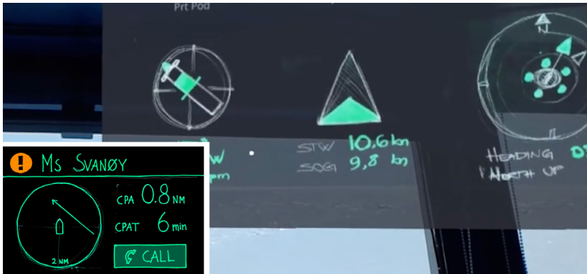
Figure 34: Scanned paper sketches and video screenshots from AR based on OpenBridge design system drawn and captured through HoloLens. (Photos: OICL)
