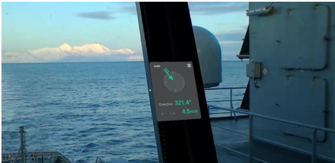
Figure 3. Examples of widgets and a container with several widgets digitally attached to various surfaces. Above, a combination of information usually found in a conning interface, displayed on the bow of the ship. Below, wind information, displayed on the surface between two windows in the aft deck.
