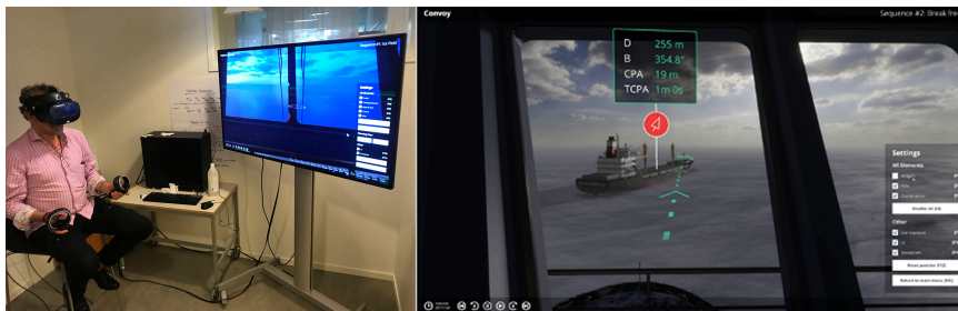
Figure 30: The Setup of the Virtual Reality-Reconstructed Operation Scenarios (VRROS). (Photo: OICL)
