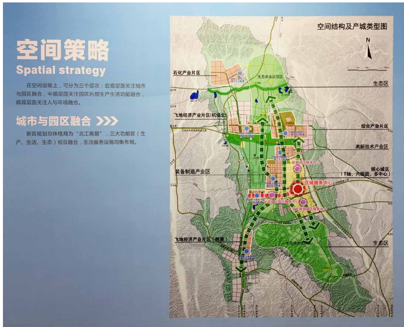
Fig. 5.5: A masterplan of Lanzhou New Area in the city’s planning bureau showroom shows the spatial layout of different land uses and institutions: The center contains government buildings and civic infrastructures for culture and leisure. It is surrounded by zones for trade and logistics, education, industries and manufacturing, the airport in the west, and petrochemical industries in the far northwest. In addition, there are zones for environmental protection and innovative agriculture in the north and south.
