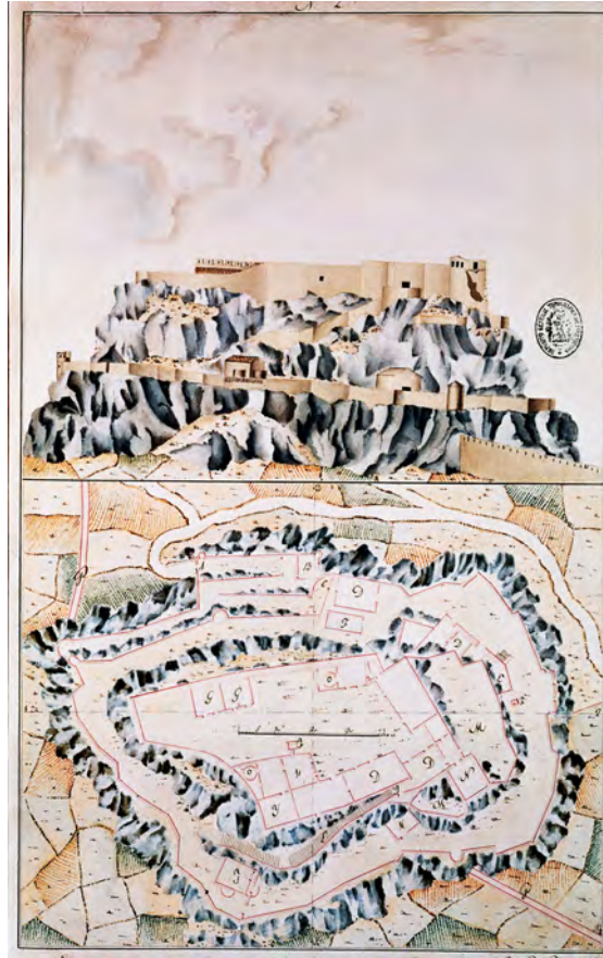
Figure 12: Fortification of Morella, where the built adapts and fusions with the terrain and its topography. It later became a village with concave-formed streets winding concentrically up the mountain (1822). Plan: Archivo Historica Militar. Madrid, Spain.
