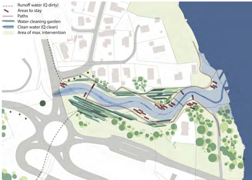
Figure 81: Water purification at Kjørbekk's outlet to Skien River. The clean water runs in the middle and on the sides; the water is slowed down and filtered through vegetation before reaching the main watercourse. Plan: Celia Martinez Hidalgo.
