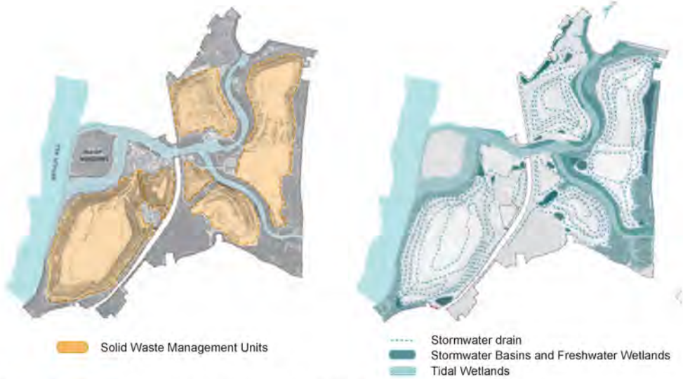
Figure 2c. Illustration of Fresh Kills. To the left, the division into four waste management units that have been elaborated in different phases. To the right, the stormwater management with runoff, stormwater basins and the tidal wetlands on the coastline. Illustration by: Celia Martinez Hidalgo (Based on the Fresh Kills Park, Project Description, 2008).
