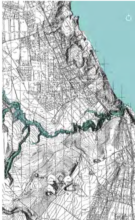
Figure 50: Historical map of the area from 1936 showing the valley of Kjørbekk before it was filled in. Single-family houses have been built to the north but no industrial activity has been installed yet. Here, the area of the sand quarry 'Nenset' to the south of Kjørbekk is seen before the sand masses were removed. Map: Municipality of Skien
