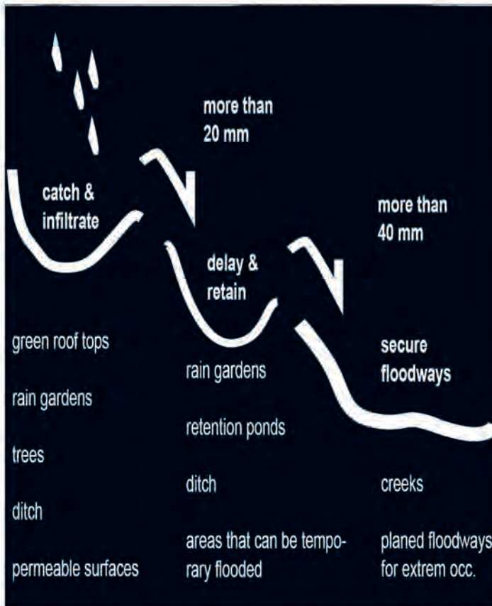
Figure 4. Illustration based on Oddvar Lindholm's SWM strategy of "The Three Step Principle", Norsk Vann Rapport R-162, p. 8. Further elaborated by Oslo Municipality SWM 2013–30, "Tre trinn prinsippet". Traced and translated by the author in 2017.
