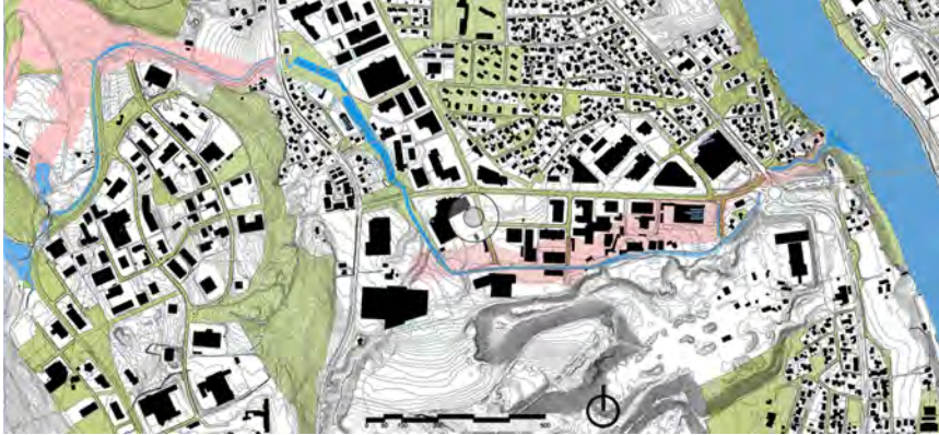
Figure 77: Landfills in pink: to the west, Kjørbekk II and to the east, Kjørbekk I. The water from the former drinking water source at Hvitsteintjern runs openly for one kilometre. It flows three kilometres in underground culverts before finally emptying into the Skien River in the east. Plan: Worksonland.
