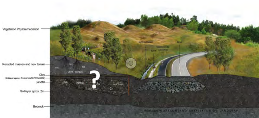
Figure 78: Sectional perspective of Kjørbekk II as an approximation of the underground of old landfill and recycled and remodelled ground. Sectional perspective: Worksonland.
